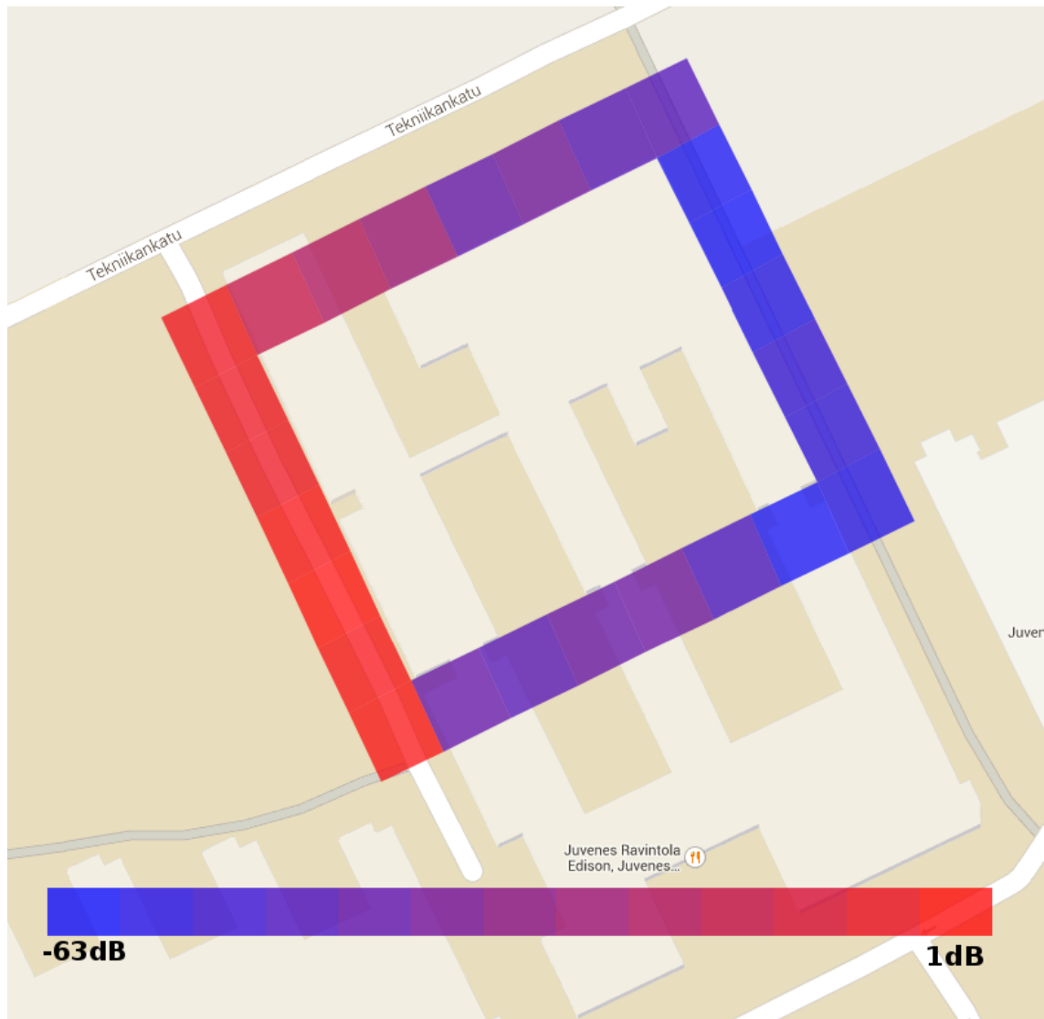
Figure 4.1 Graphical representation of the results, AFRCN 93: 956,3MHz
