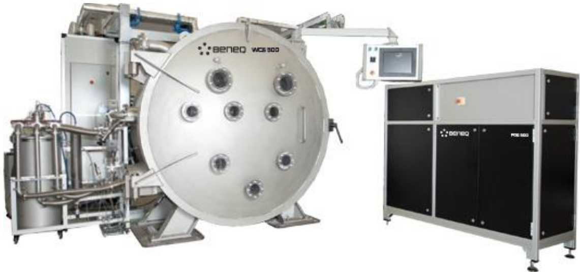
Figure 3.1. Roll-to-Roll ALD device WCS 500 by Beneq [12]
