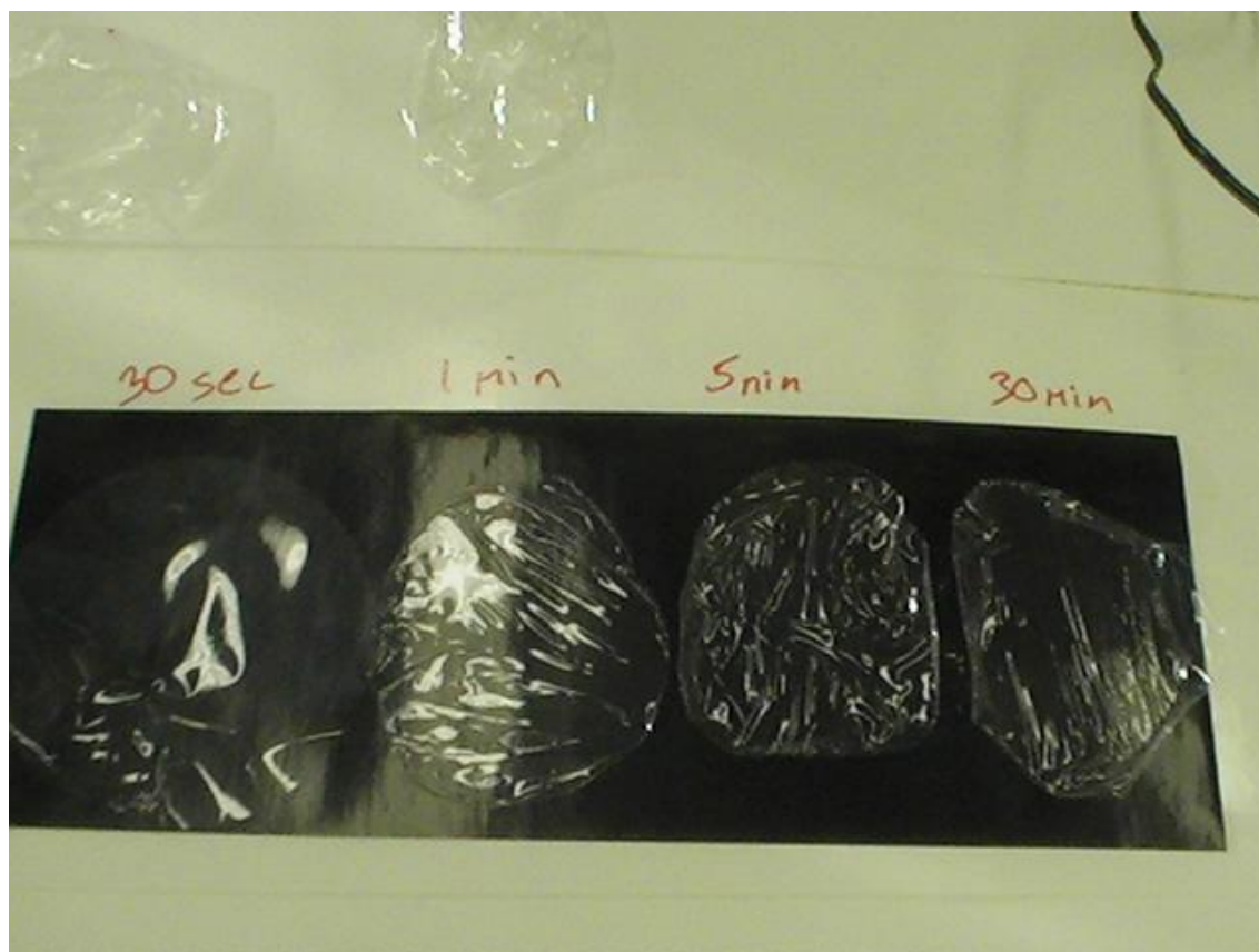
Figure 5.3.3. PLA films kept in an oven at 100°C for a period of time written above the samples.
