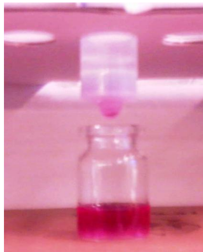
Figure 22: Elution phase of Immobilized Metal Affinity Chromatography (IMAC). His-KR protein was collected in a vial placed under IMAC column
