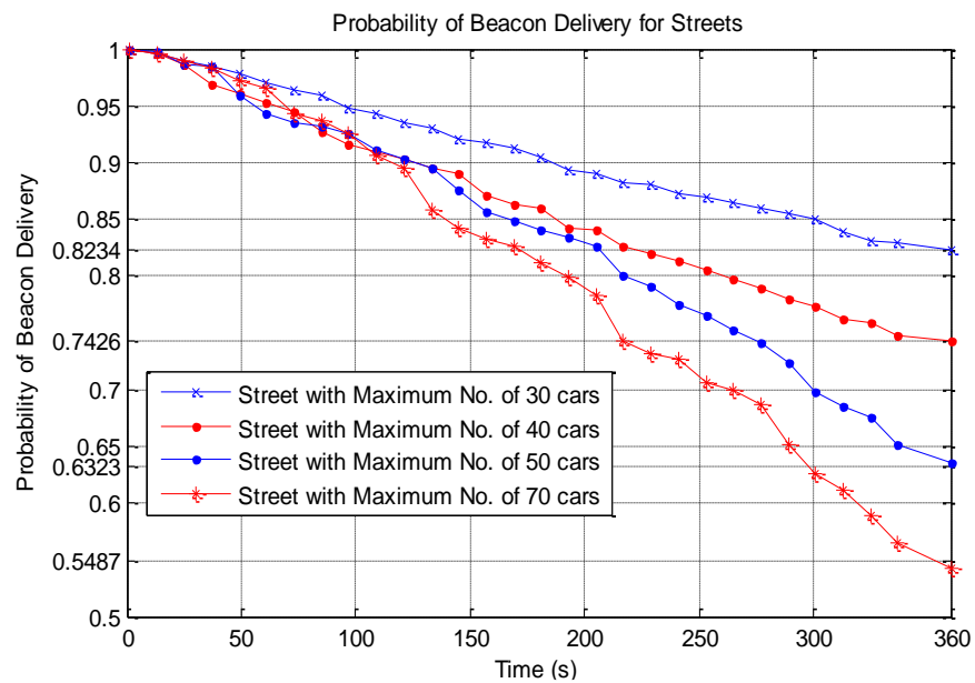
Figure 4-6. Probability of Beacon Delivery for Different Streets with different Number of Cars.
