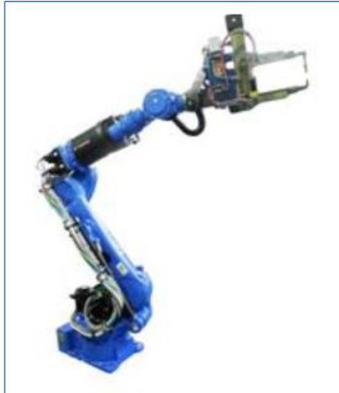
Figure 4-31 Motoman MS210 spot welding robot.
