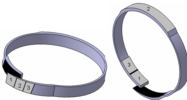
Figure 26 Schematic for the electrode placement of the ECG bracelet
