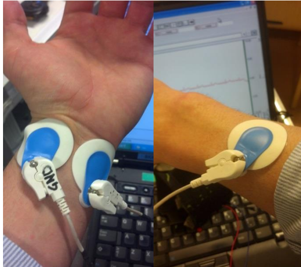
Figure 34 Ag/AgCl electrode placement on left and right hands while connected to the Biopac MP36
