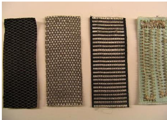
Figure 22 Different types of electrodes used in ECG measurement. The first three electrodes were made industrially but the fourth electrode is the handmade embroidered conductive yarn [40]
