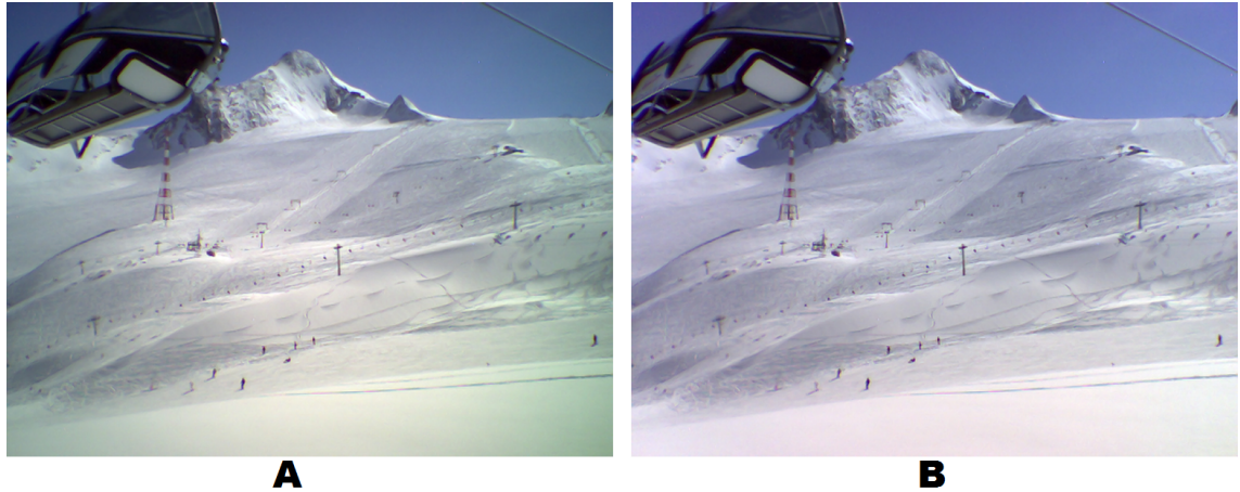
Figure 2.11: Example of an image without (A) and with (B) vignetting correction [13].
