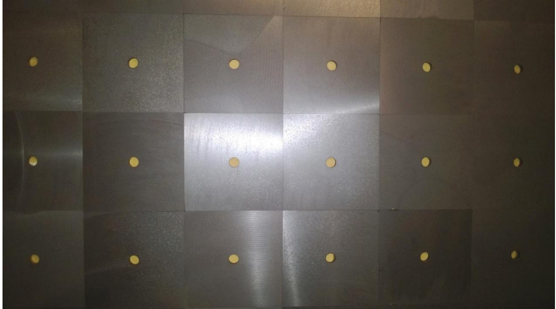
Figure 3.3 ferrite tiles lined on the inner walls of TUT's chamber
