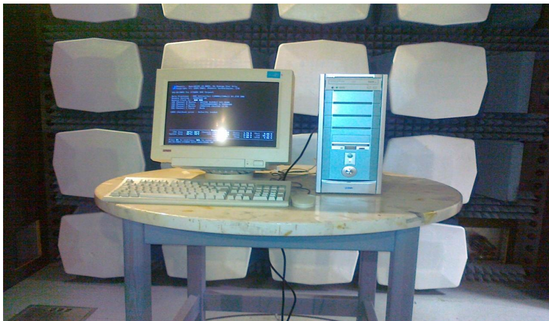
Figure 4.9 Equipment under test (computer) for radiated emission test
