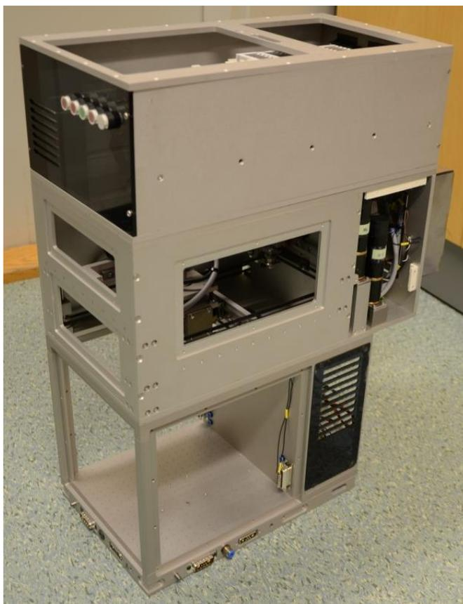
**Figure 5-1 Physical prototype of the TUT  $\mu$ F cell consisting from base module, process module (DOHMAN) and control and vision module**
