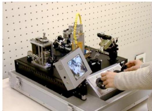
Figure 1-1 Micro-lathe (left) [3]; Portable microfactory (right) [3] [4]
