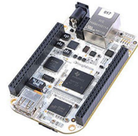
b) BeagleBone [23], an ARM Cortex-A8 based embedded Linux platform.
