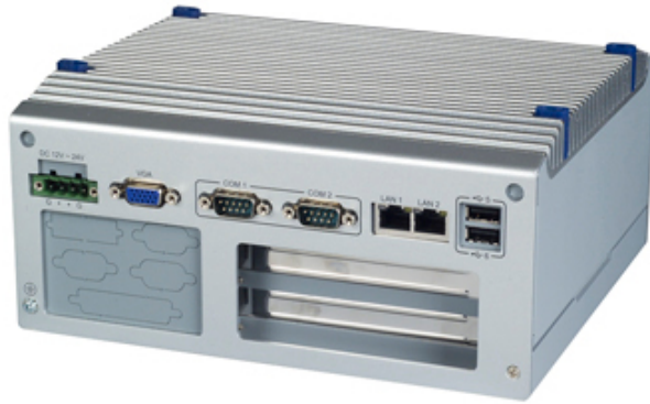
a) Advantech ARK-3403 [26], an Intel Atom based embedded Windows PC.
