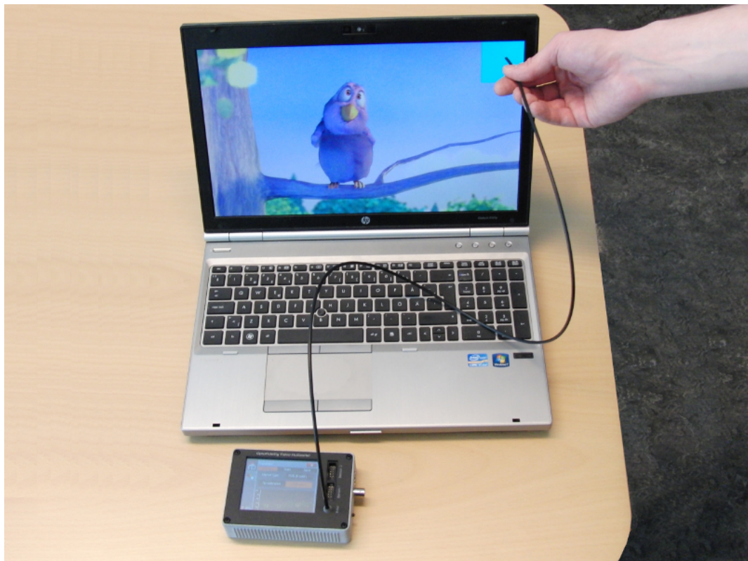
Figure 1.2: An example measurement setup where the video playback performance of a laptop computer is being measured.
