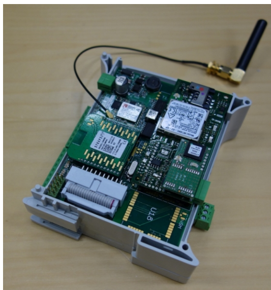
Figure 3.6: 6LoWPAN expansion module for the S1000 RTU
