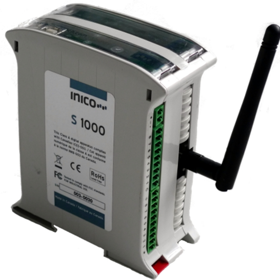
Figure 3.5: Inico S1000 RTU and its wireless expansion
