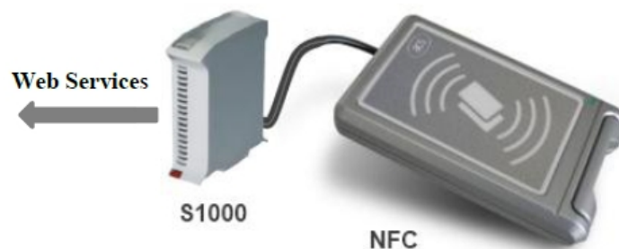
Figure 3.14: NFC reader connected to the Inico S1000 RTU
