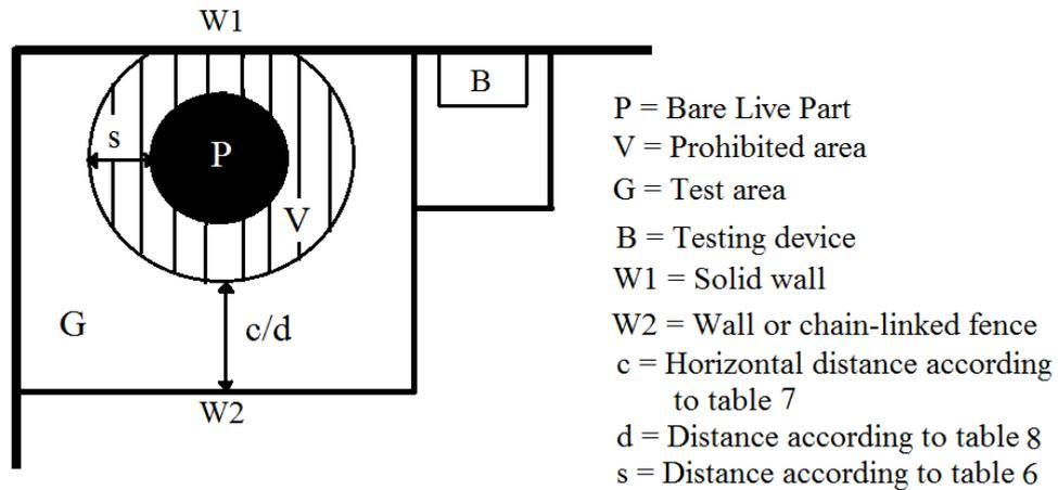
**Figure 4.** Example of different areas of a test station [14]
