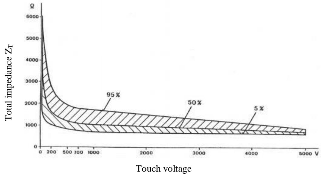
**Figure 2.** Total impedance of a human body in function of touch voltage. [1]
