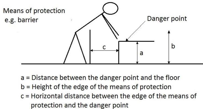
**Figure 5.** Demonstration of the dimensions listed in Table 14. [14]
