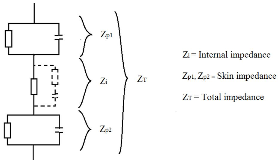
*Figure 1. Total impedance of a human body [1].*
