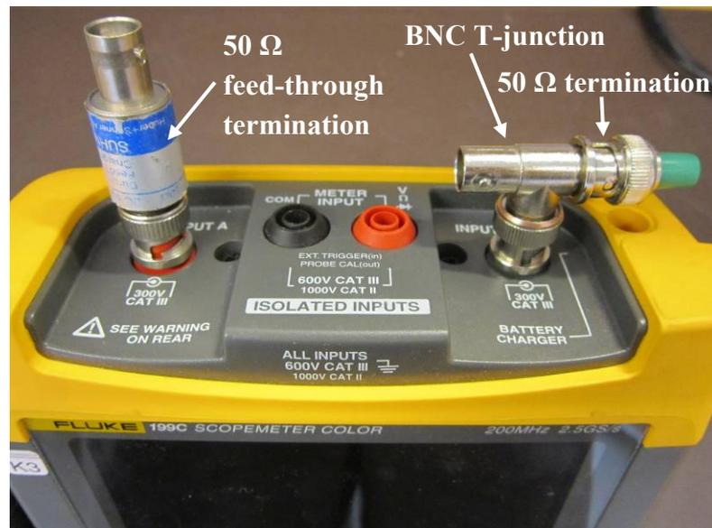
**Figure 4.7** 50  $\Omega$  feed-through termination and 50  $\Omega$  T-termination in the oscilloscope's high impedance inputs.
