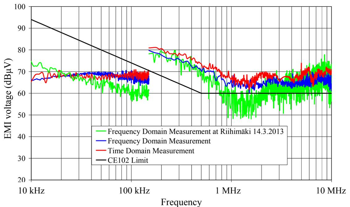
**Figure 8.3** TDEMI measurement results and frequency domain EMI measurement results, DC-motor of the reference EMI source, return lead.
