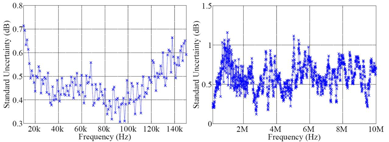
**Figure 6.8** The standard uncertainty of the measurement results, interference signal from DC motor.
