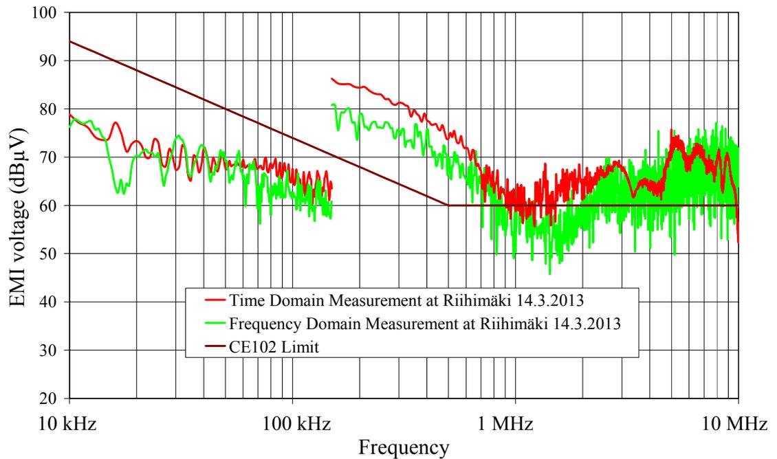
**Figure 8.4** TDEMI measurement results and frequency domain EMI measurement results, both measurements at Riihimäki 14.3.2013, DC-motor of the reference EMI source, plus lead.
