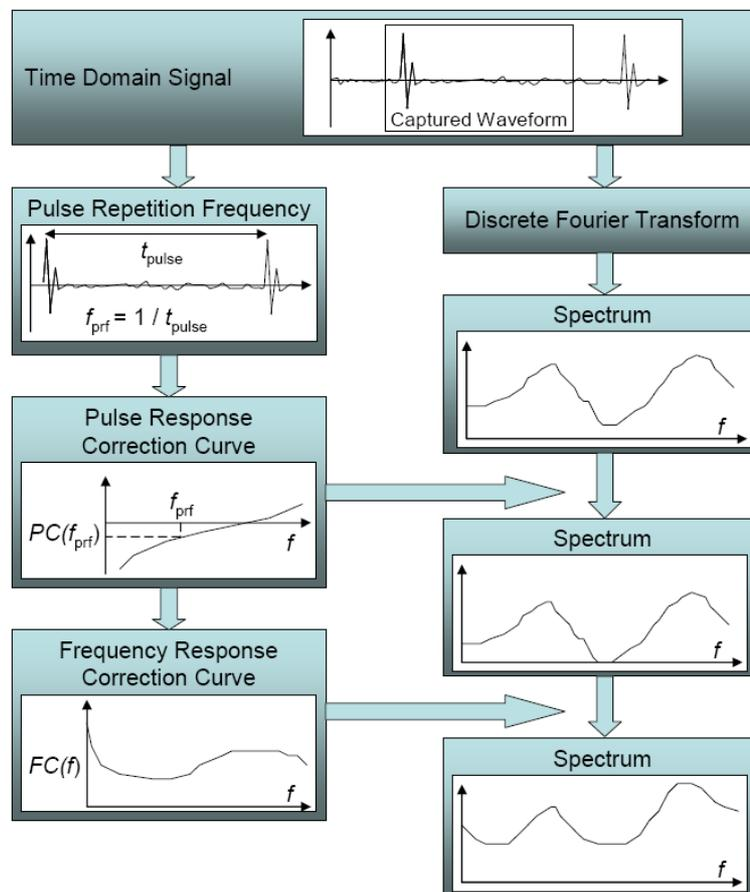
**Figure 1.6** Algorithm for correction of broadband interference [7].
