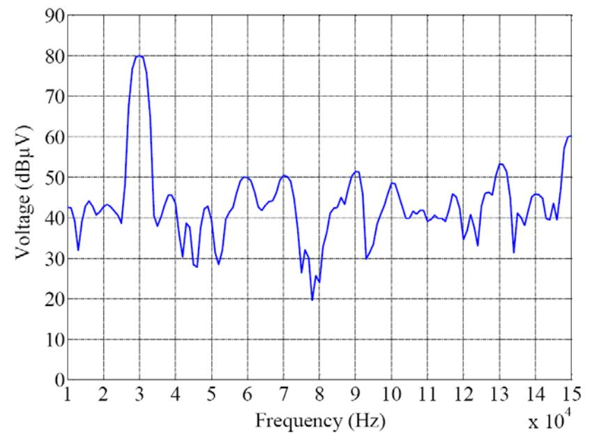
Amplitude spectrum of a 30.5 kHz sinusoidal signal without Flat Top windowing before DFT
