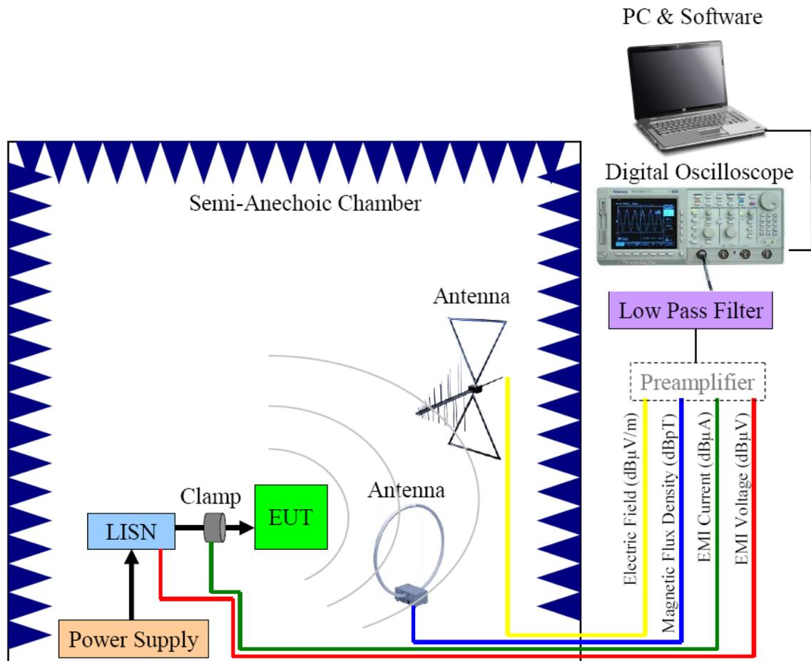
**Figure 1.2** Example of time domain EMI measurement system.
