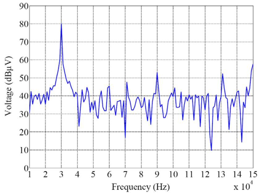
Amplitude spectrum of a 30 kHz sinusoidal signal with Flat Top windowing before DFT. Coherent gain included.
