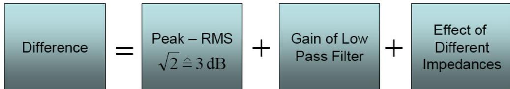
*Figure 4.11 The reasons for the difference between frequency and time domain measurements.*
