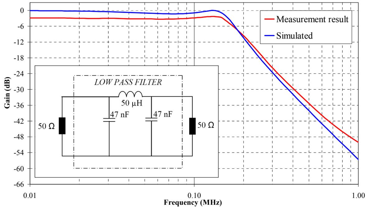
**Figure 4.4** Circuit, simulated and measured frequency responses of low pass filter #1.
