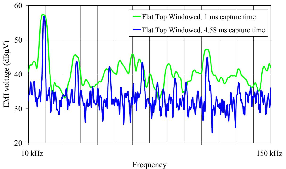
**Figure 5.9** The effect of longer capture time. Interference signal from the DC/DC converter of the reference EMI source.
