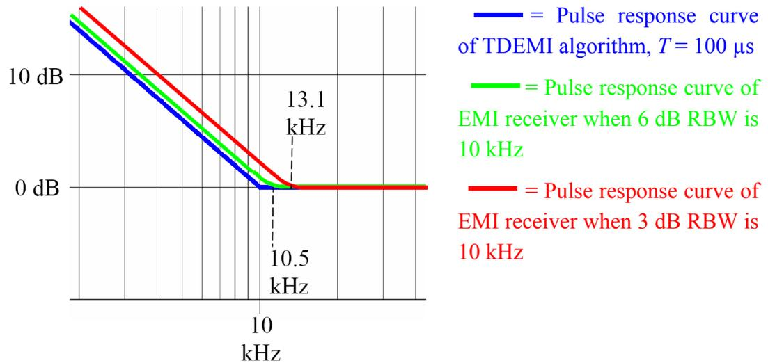
**Figure 5.17** Pulse response curves in the vicinity of 10 kHz.
