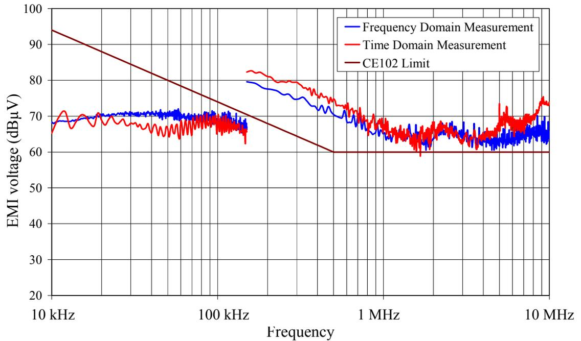
**Figure 4.15** TDEMI measurement results compared to frequency domain EMI measurement results, DC-motor of reference EMI source, plus lead.
