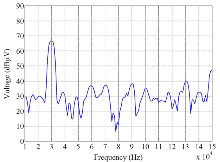
Amplitude spectrum of a 30 kHz sinusoidal signal with Flat Top windowing before DFT. Coherent gain compensated.
