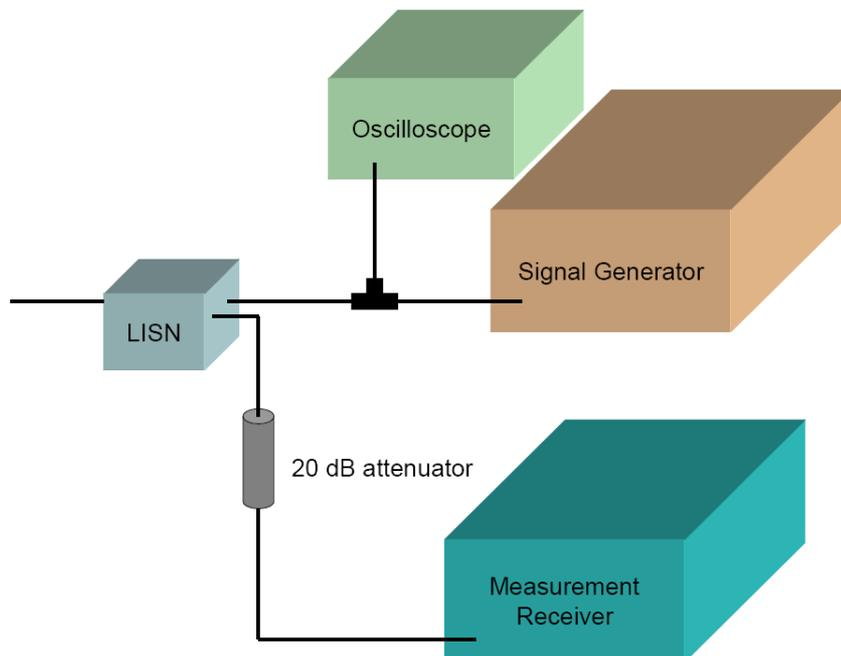
*Figure 3.4 CE102 measurement setup calibration.*
