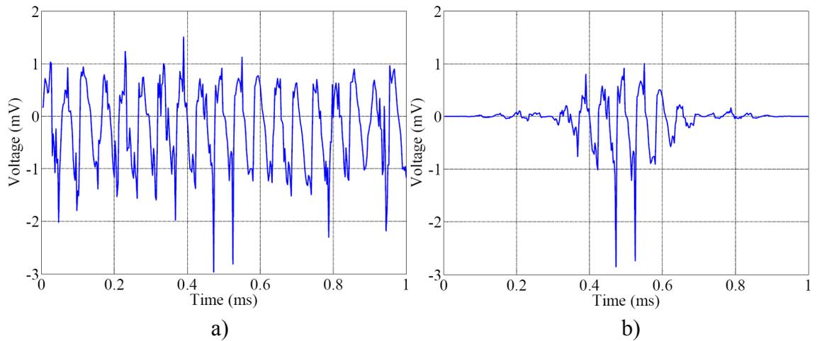
**Figure 5.5 a)** Interference signal caused by DC/DC converter of reference EMI source, capture time 1 ms **b)** Same signal after Flat Top windowing.
