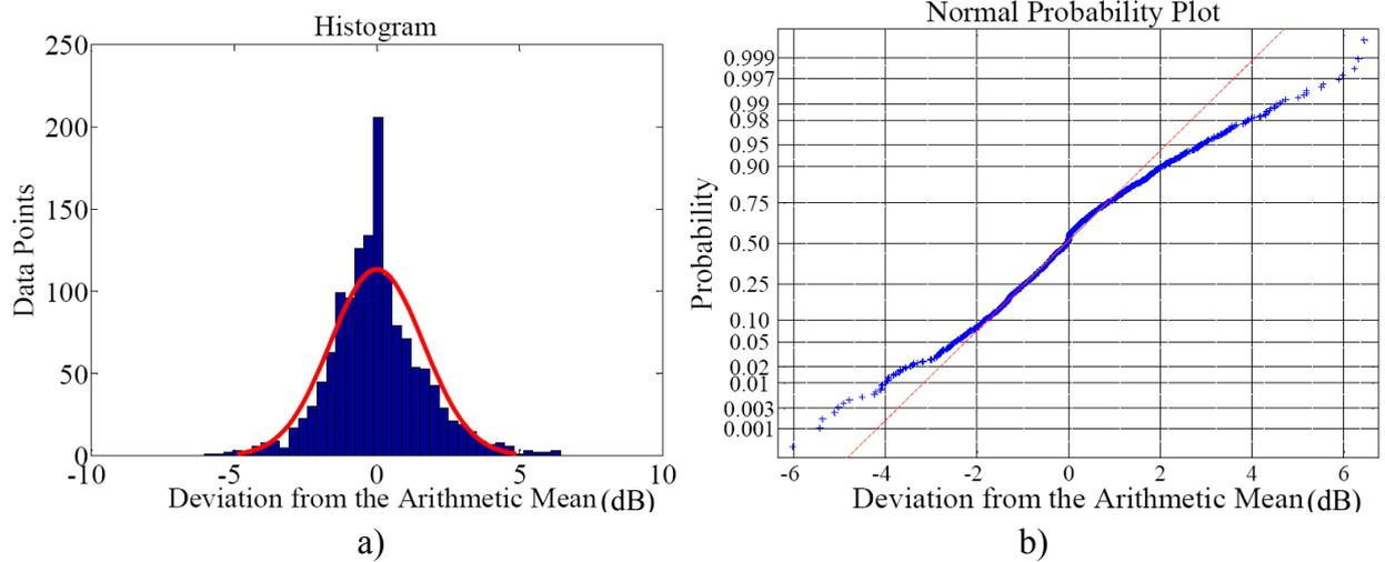
**Figure 6.6 a)** Histogram of individual measurement results, 10 kHz - 150 kHz / 2820 data points **b)** Normal probability plot of individual measurement results, 10 kHz - 150 kHz / 2820 data points.
