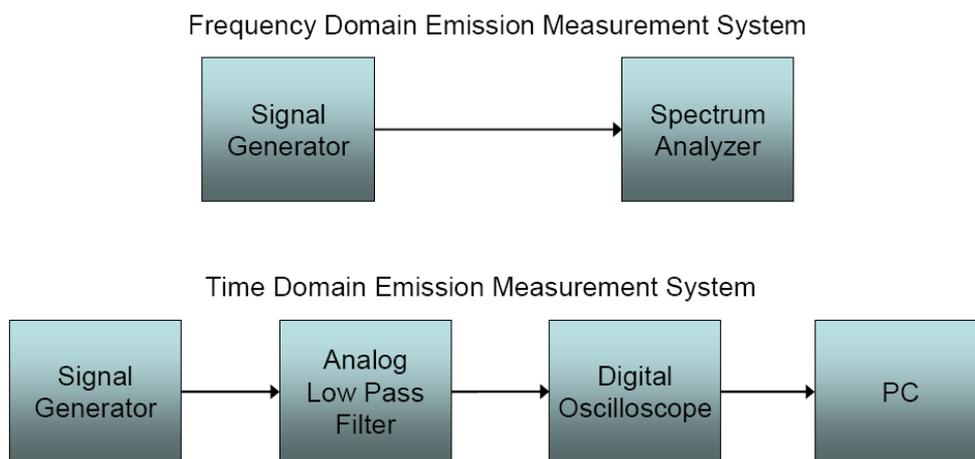
**Figure 4.8** Measurement setups used in correction determination.
