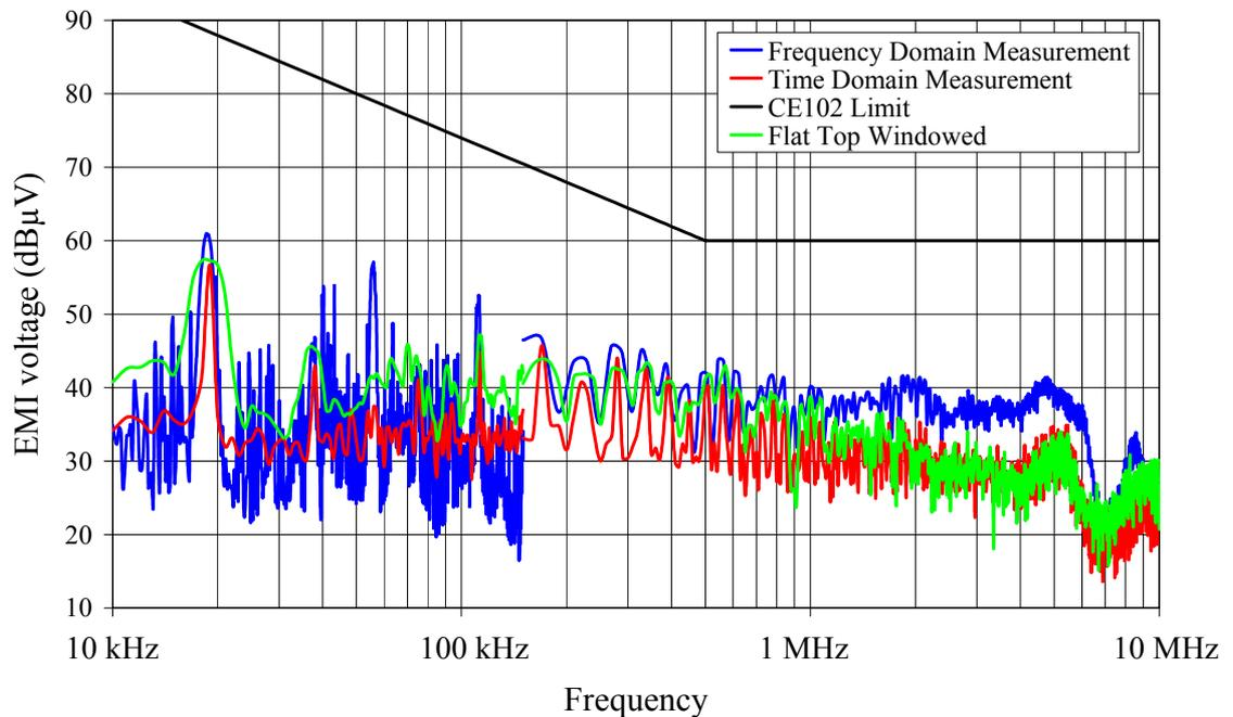
**Figure 5.7** TDEMI measurement results compared to frequency domain EMI measurement results, DC/DC converter of reference EMI source, plus lead.
