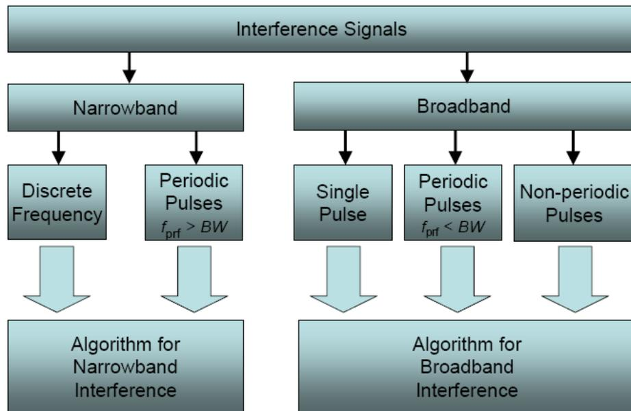
**Figure 1.4** Interference classifications [7].
