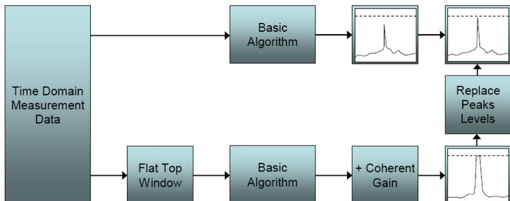
**Figure 1.5** Algorithm for correction of narrowband interference i.e. peaks [7].
