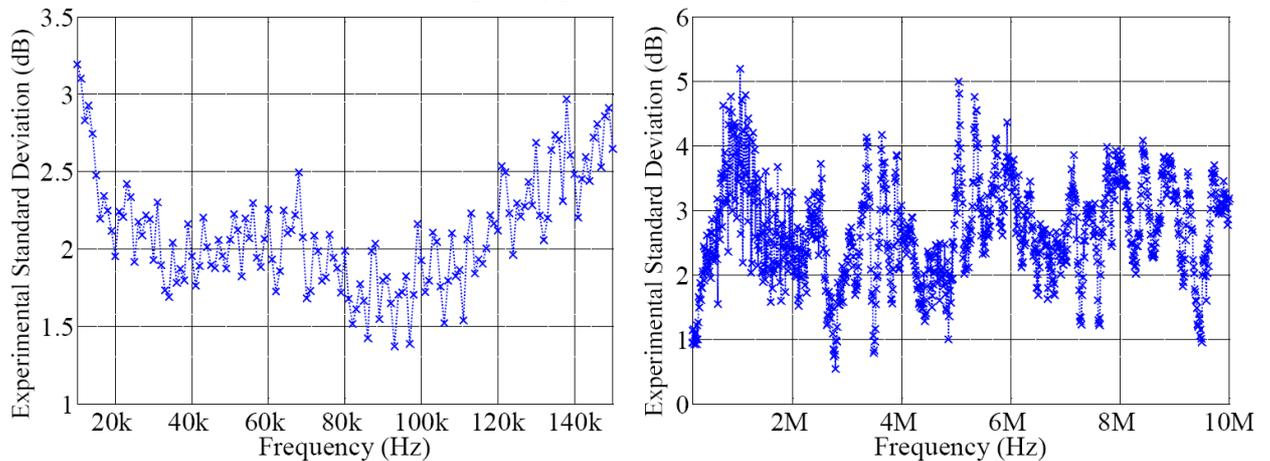
**Figure 6.7** The experimental standard deviation of the measurement results, interference signal from DC motor.
