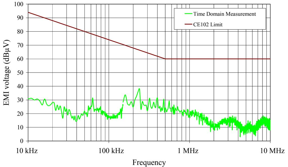
**Figure 4.12** Ambient electromagnetic interference, plus lead.
