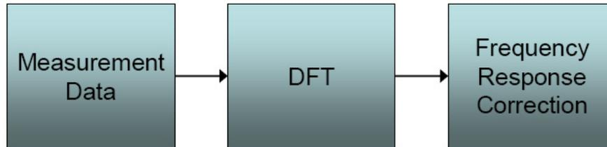
*Figure 4.1 Basic algorithm for time domain emission measurement system.*
