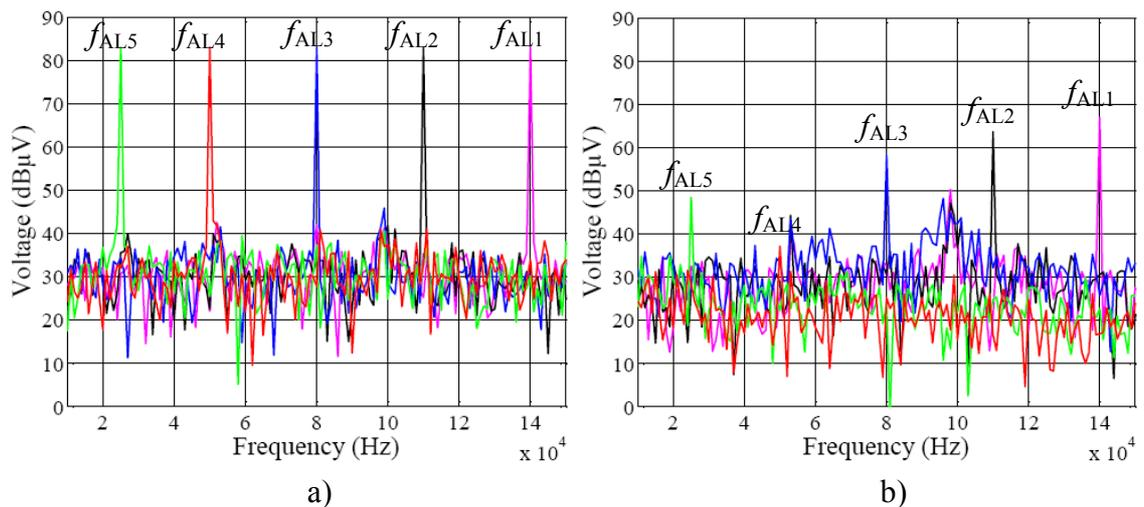
**Figure 4.8** Aliased test signals a) without low pass filter #1 and b) with low pass filter #1.
