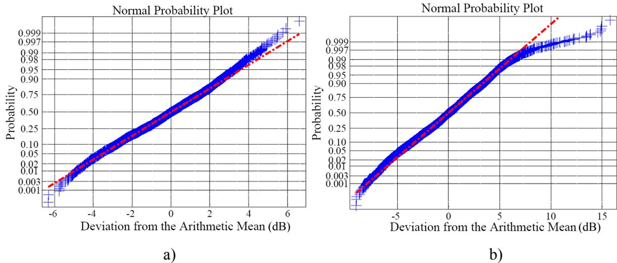
**Figure 6.10 a)** Normal probability plot of individual measurement results, 10 kHz - 150 kHz / 2820 data points **b)** Normal probability plot of individual measurement results, 150 kHz - 10 MHz / 19720 data points.
