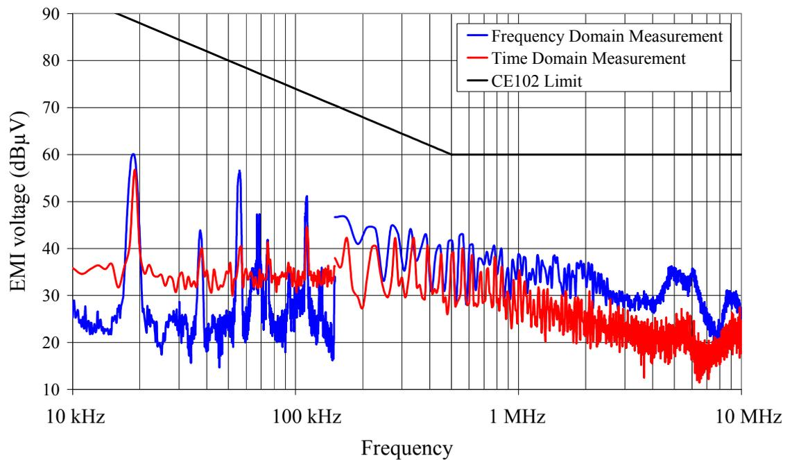
**Figure 4.14** TDEMI measurement results compared to frequency domain EMI measurement results, DC/DC converter of reference EMI source, return lead.
