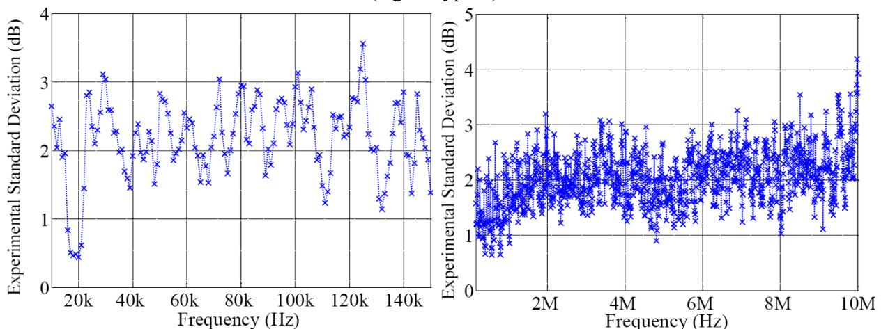
**Figure 6.1** The experimental standard deviation of the measurement results, interference signal from DC/DC converter.
