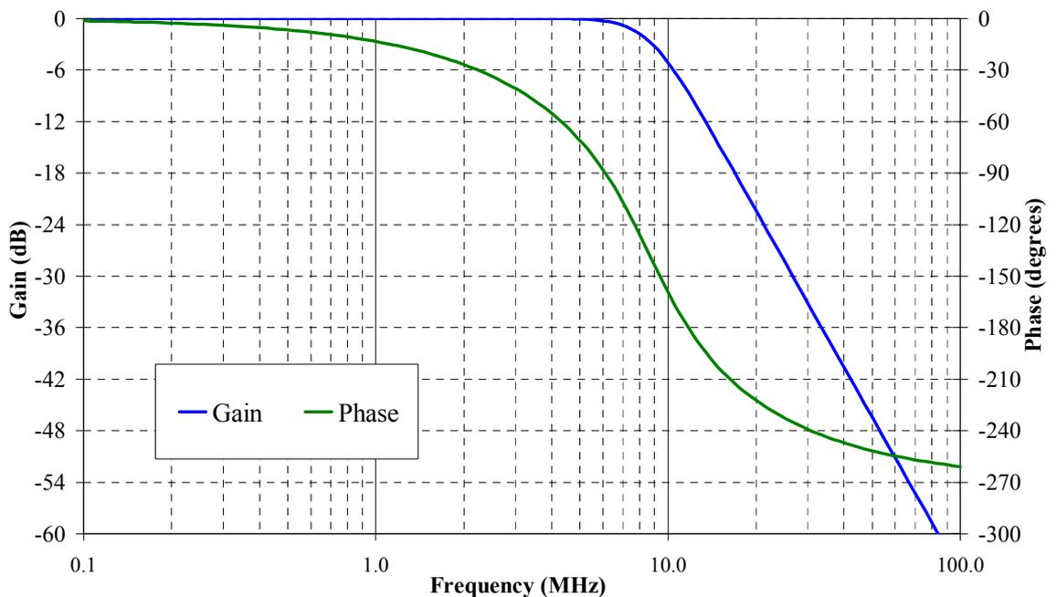
**Figure 4.7** Simulated gain and phase of low pass filter #2.
