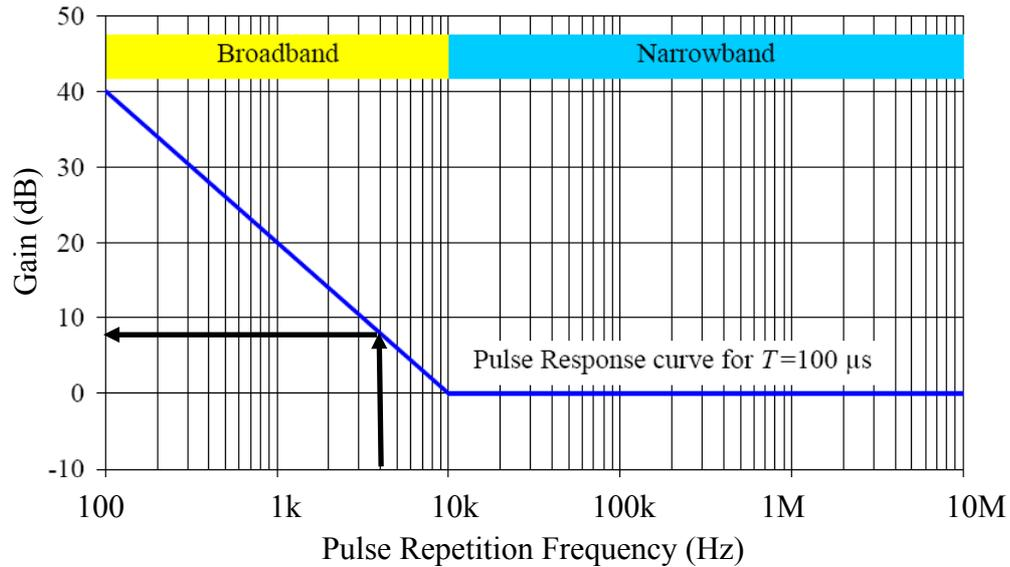
**Figure 5.14** Pulse response curve of TDEMI algorithm, capture time  $T = 100 \mu\text{s}$ , response for the 4 kHz signal is shown with the arrows.
