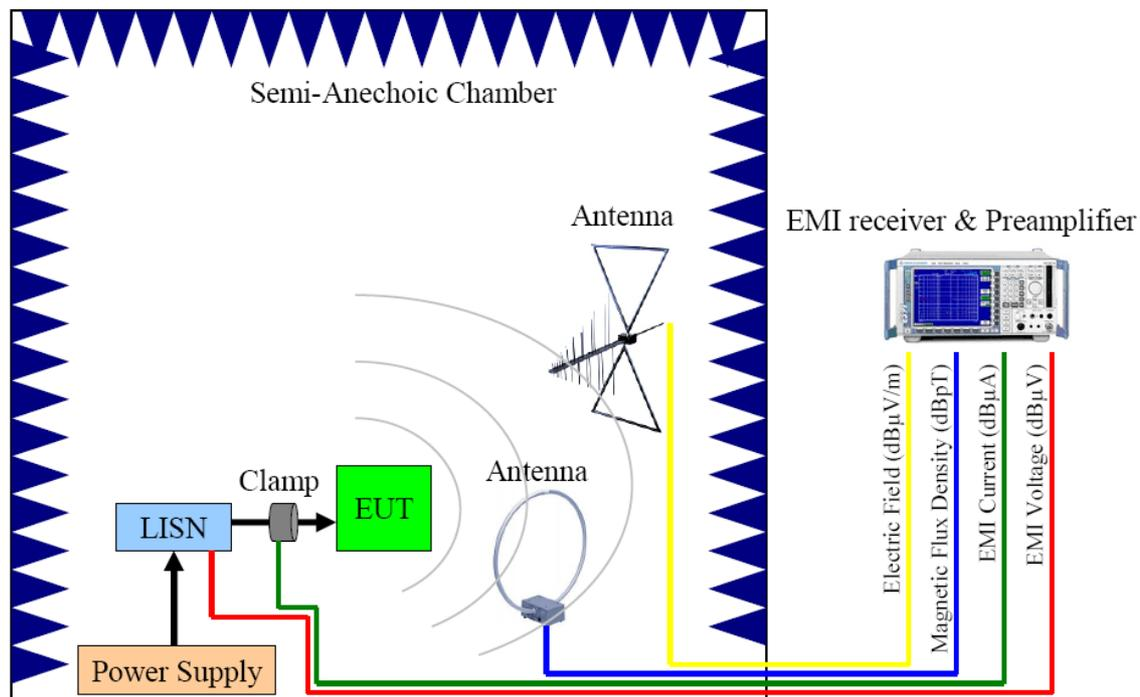
**Figure 1.1** Example of frequency domain EMI measurement system.
