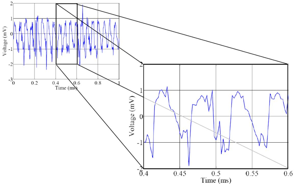
**Figure 5.4** Differential mode interference voltage caused by DC/DC converter of reference EMI source.
