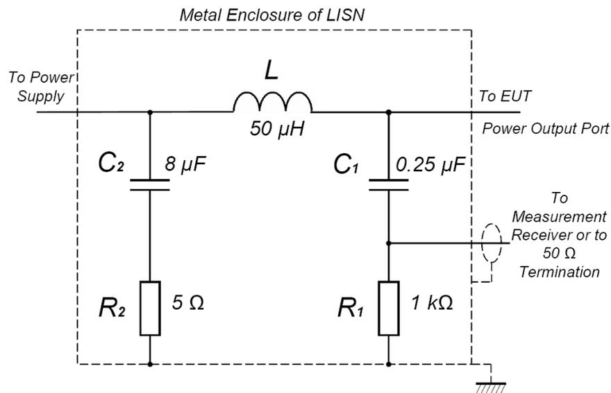
**Figure 3.1** MIL-STD-461F LISN circuit schematics.
