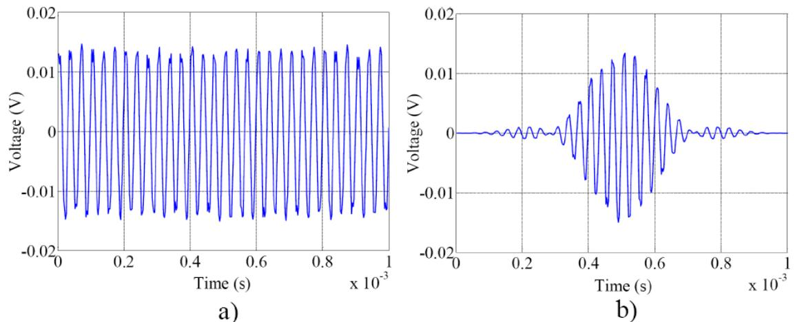
**Figure 5.2** Captured 30.5 kHz test signal **a)** before windowing **b)** after windowing with Flat Top window function.
