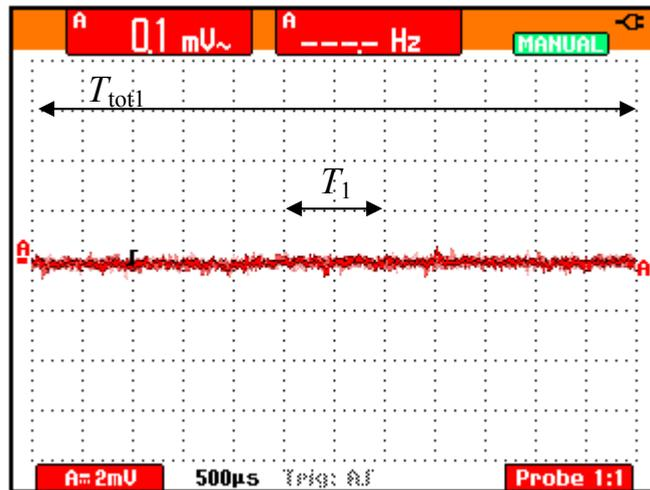
**Figure 4.2** Total capture time  $T_{tot1}$  and capture time  $T_1$  on frequency range from 10 kHz to 150 kHz.  $T_1$  can be chosen arbitrarily from the  $T_{tot1}$ .
