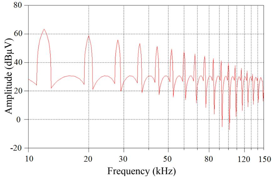
**Figure 5.11** Spectrum of a 4 kHz square wave signal. Simulated TDEMI measurement result for lower frequency band (10 kHz – 150 kHz).
