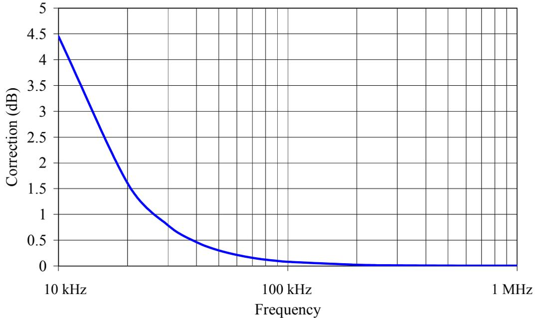
**Figure 3.5** Correction for 0.25  $\mu\text{F}$  capacitor.
