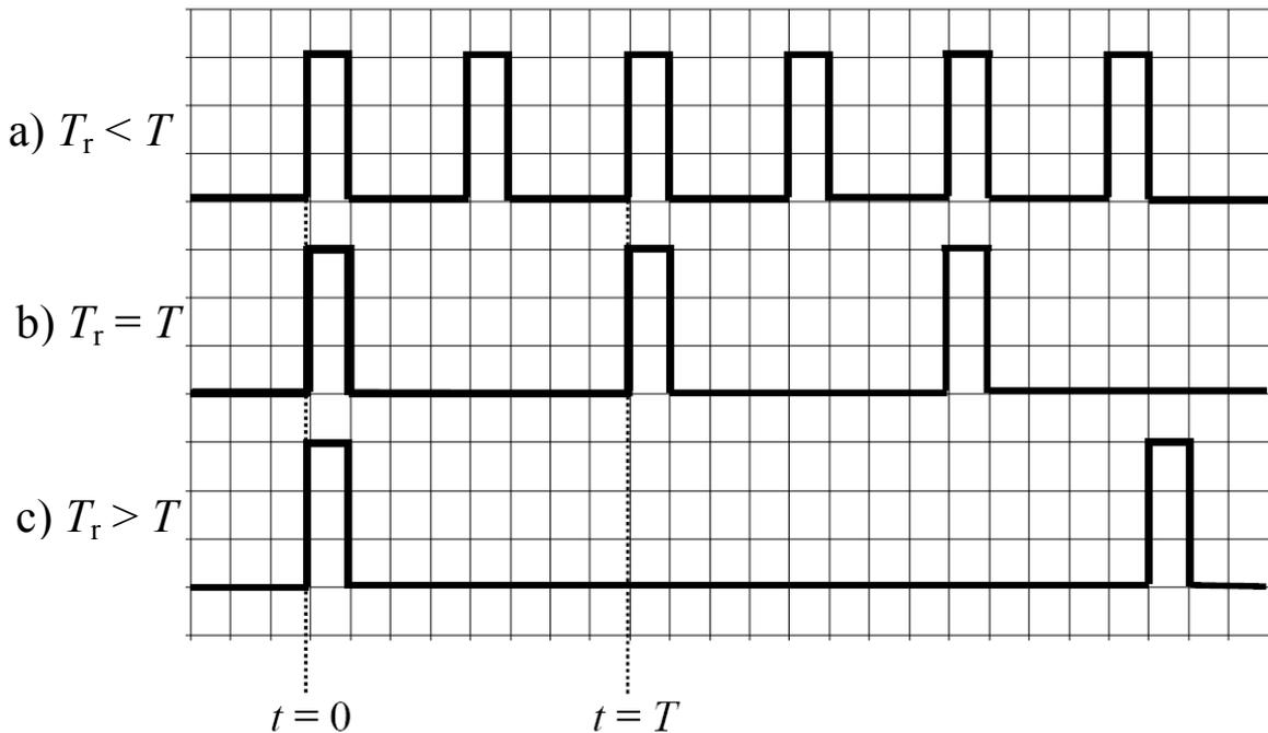
**Figure 5.13** Pulses with different repetition periods  $T_r$  and the capture time  $T$ .
