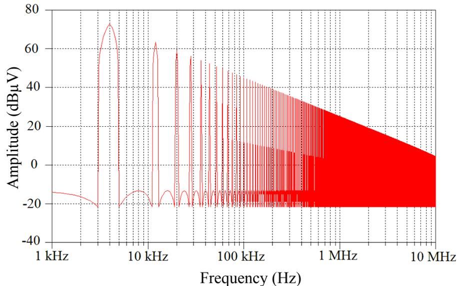
**Figure 5.10** Spectrum of a 4 kHz square wave signal.
