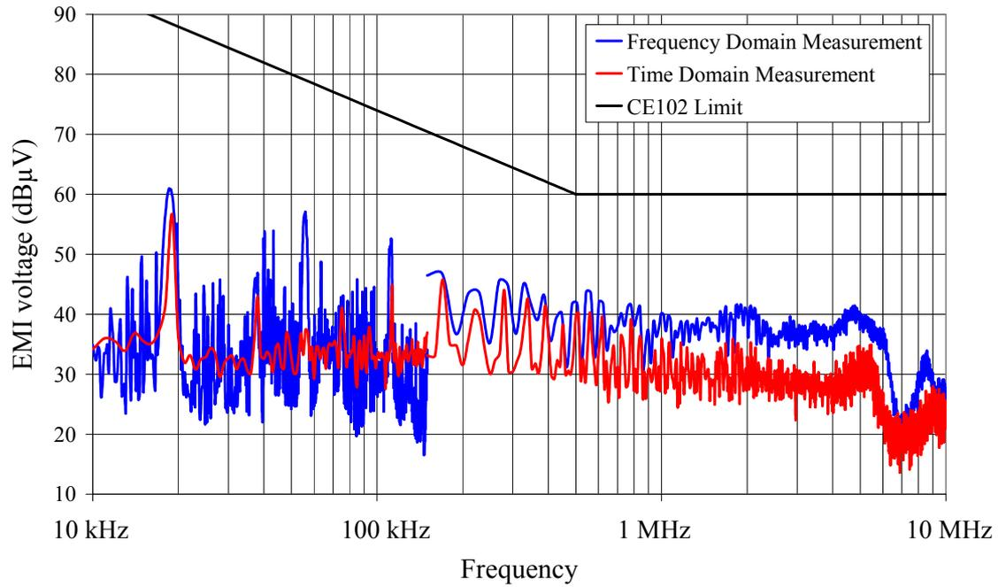
**Figure 4.13** TDEMI measurement results compared to frequency domain EMI measurement results, DC/DC converter of reference EMI source, plus lead.
