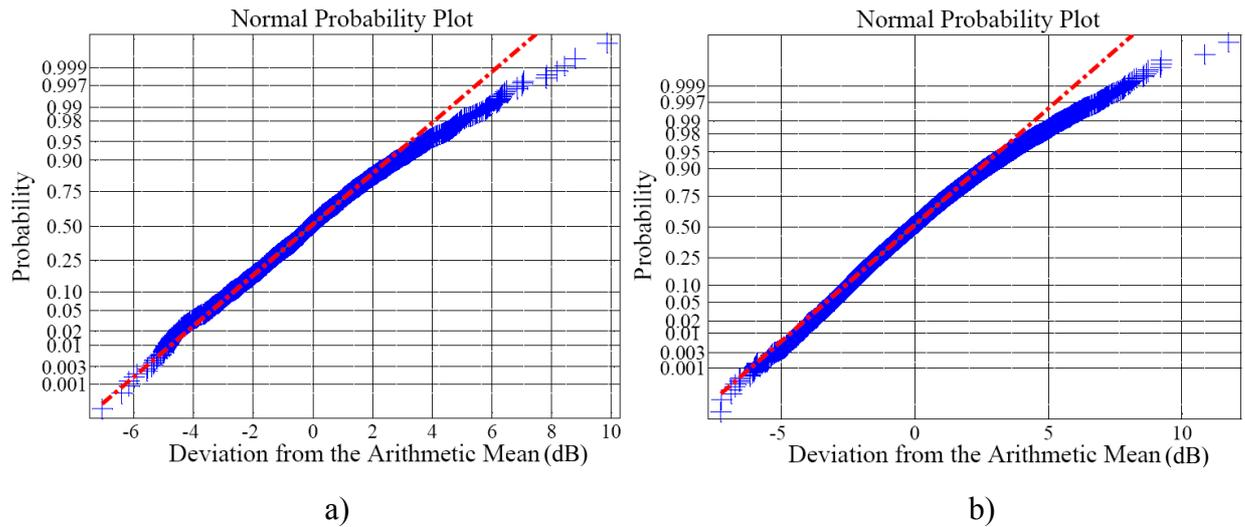
**Figure 6.4 a)** Normal probability plot of individual measurement results, 10 kHz - 150 kHz / 2820 data points **b)** Normal probability plot of individual measurement results, 150 kHz - 10 MHz / 19720 data points.
