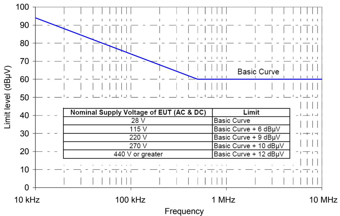
**Figure 3.3** MIL-STD-461F limit levels for CE102 measurement.
