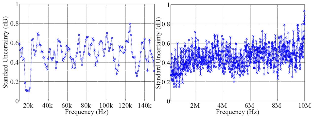
**Figure 6.2** The standard uncertainty of the measurement results, interference signal from DC/DC converter.
