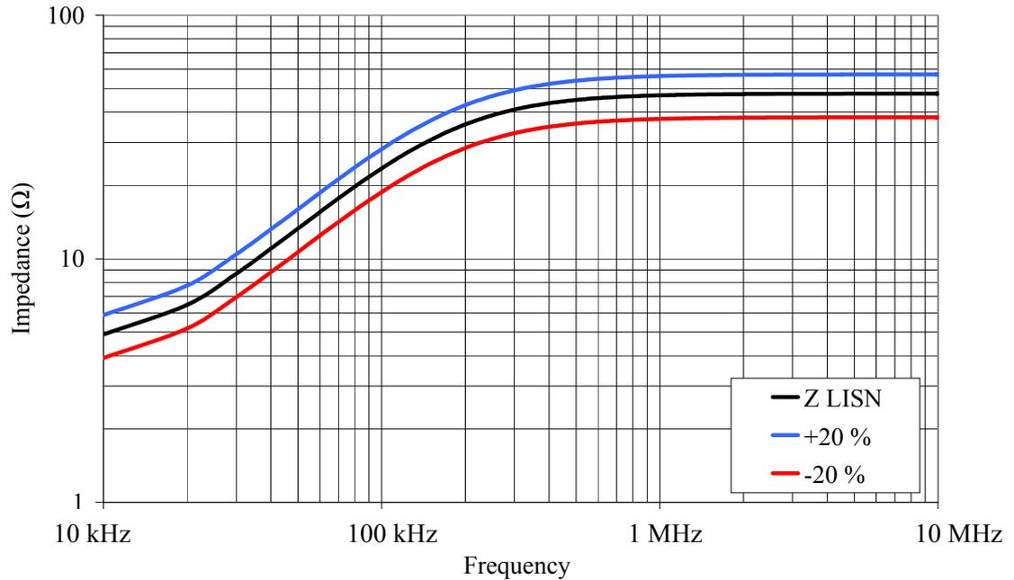
**Figure 3.2** MIL-STD-461F requirement for LISN impedance with allowed  $\pm 20\%$  tolerances.
