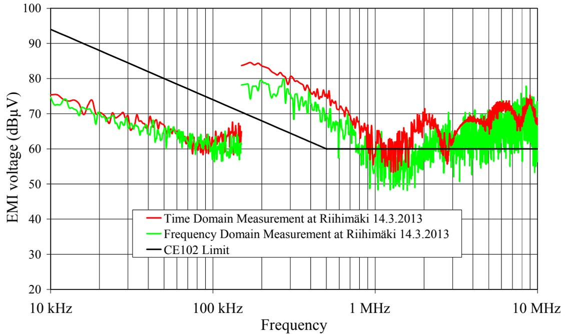
**Figure 8.5** TDEMI measurement results and frequency domain EMI measurement results, both measurements at Riihimäki 14.3.2013, DC-motor of the reference EMI source, return lead.
