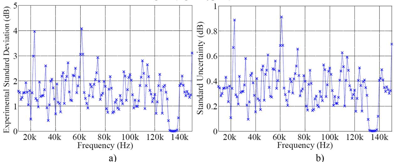
**Figure 6.5 a)** The experimental standard deviation of the discrete 135 kHz sinusoidal signal **b)** Standard uncertainty of the discrete 135 kHz sinusoidal signal.
