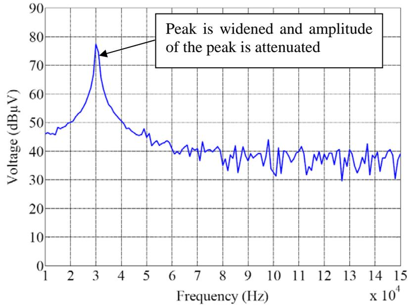
Amplitude spectrum of a 30.5 kHz sinusoidal signal with Flat Top windowing before DFT. Coherent gain included.
