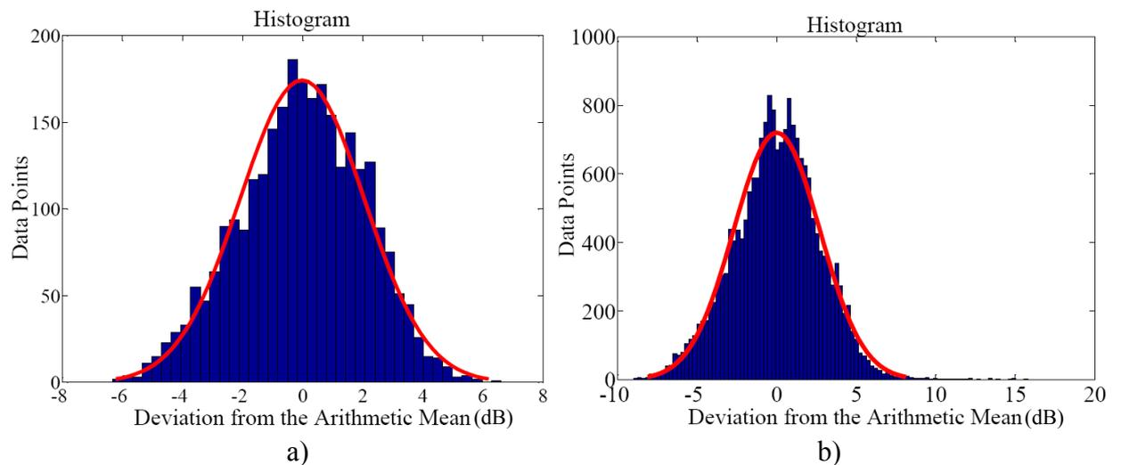
**Figure 6.9 a)** Histogram of individual measurement results, 10 kHz - 150 kHz / 2820 data points **b)** Histogram of individual measurement results, 150 kHz - 10 MHz / 19720 data points.
