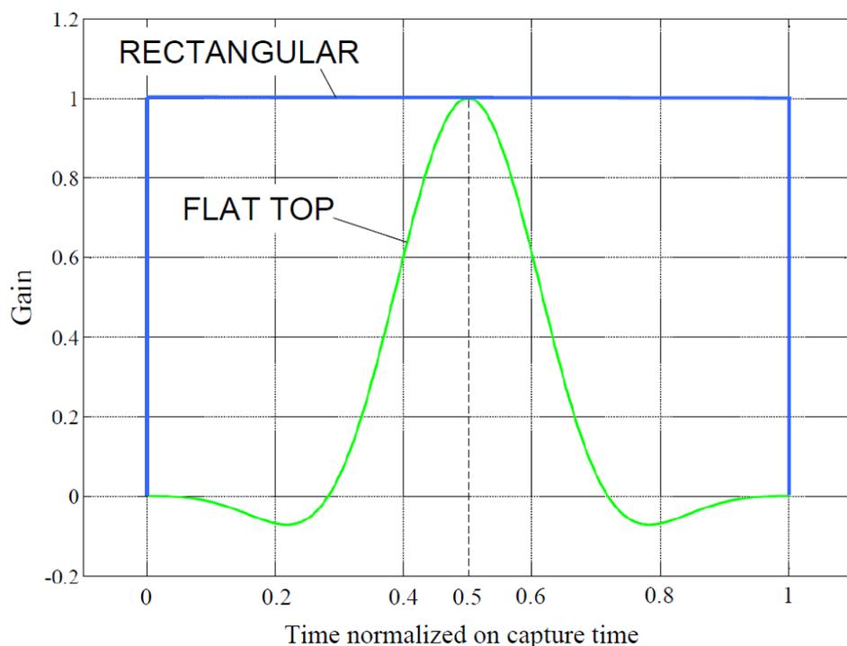
**Figure 5.1** Rectangular and Flat Top window functions.
