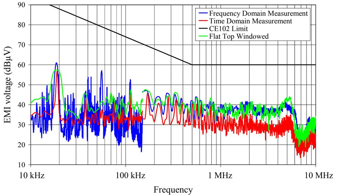
**Figure 5.8** TDEMI measurement results compared to frequency domain EMI measurement results, DC/DC converter of reference EMI source, plus lead, Flat Top windowing applied to six overlapped time domain signals (see Appendix 4).
