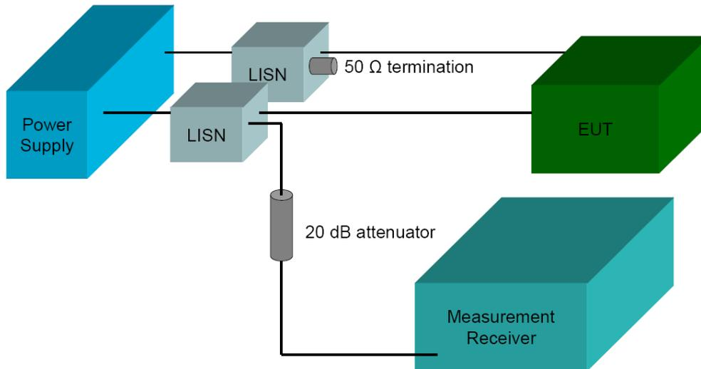
**Figure 3.6** CE102 measurement setup.
