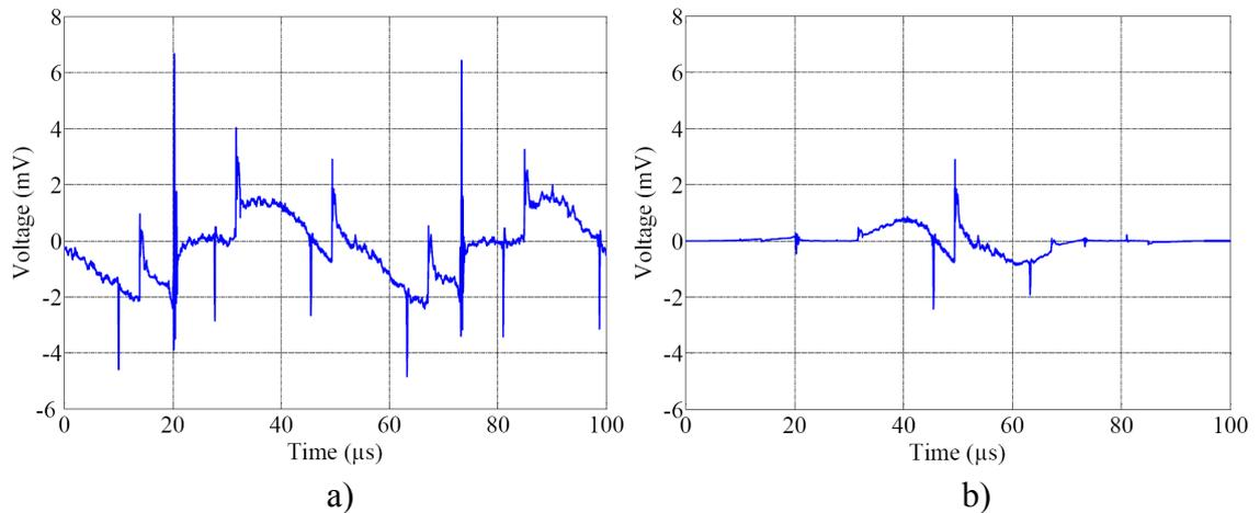
**Figure 5.6 a)** Interference signal caused by DC/DC converter of reference EMI source, capture time 100 μs **b)** Same signal after Flat Top windowing.
