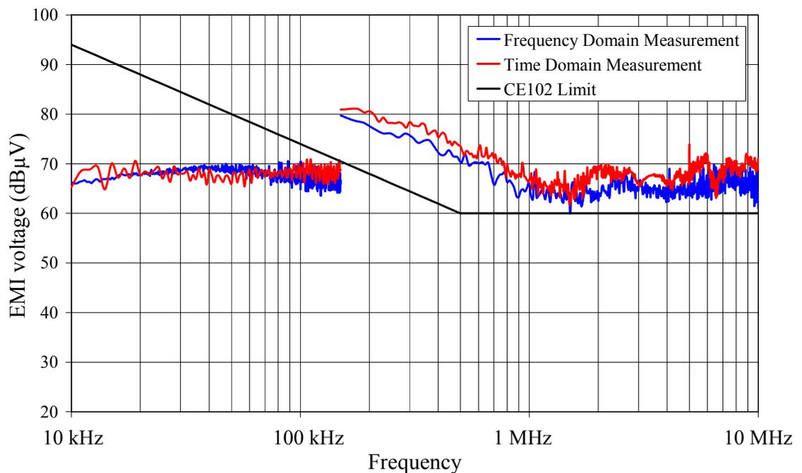
**Figure 4.16** TDEMI measurement results compared to frequency domain EMI measurement results, DC-motor of reference EMI source, return lead.
