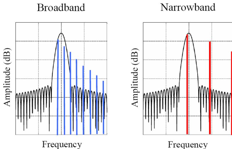
**Figure 5.15** Broadband and narrowband signals in the frequency domain.
