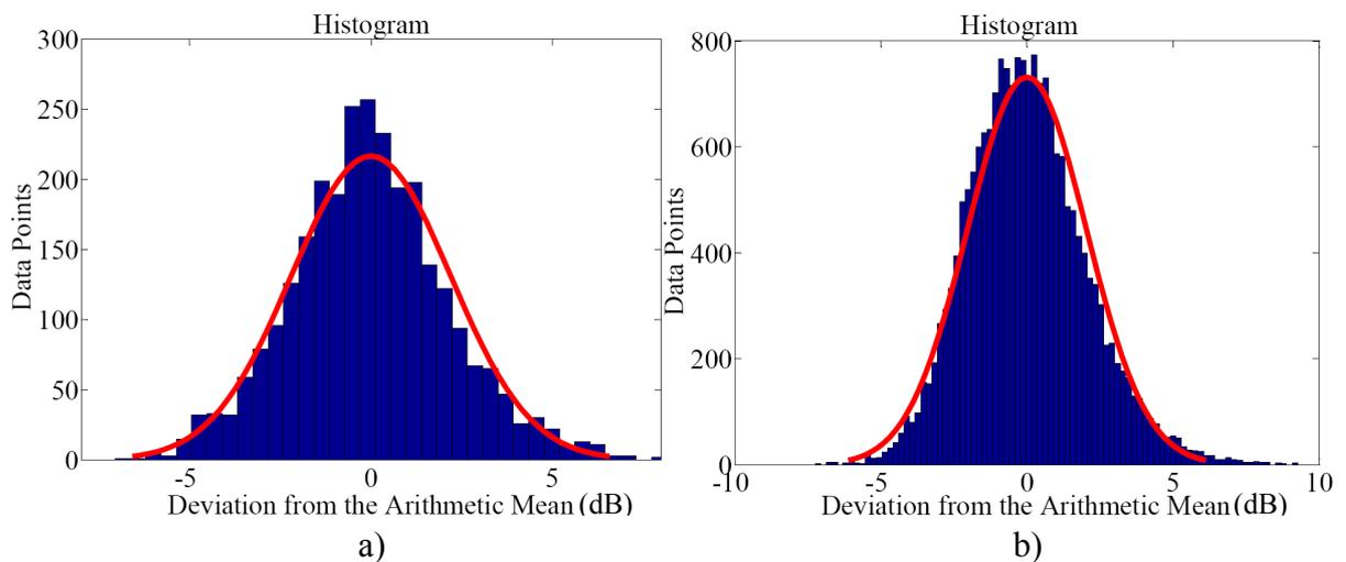
**Figure 6.3 a)** Histogram of individual measurement results, 10 kHz - 150 kHz / 2820 data points **b)** Histogram of individual measurement results, 150 kHz - 10 MHz / 19720 data points.
