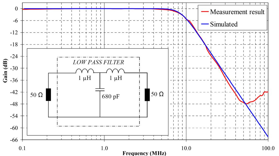
**Figure 4.5** Circuit, simulated and measured frequency responses of low pass filter #2.
