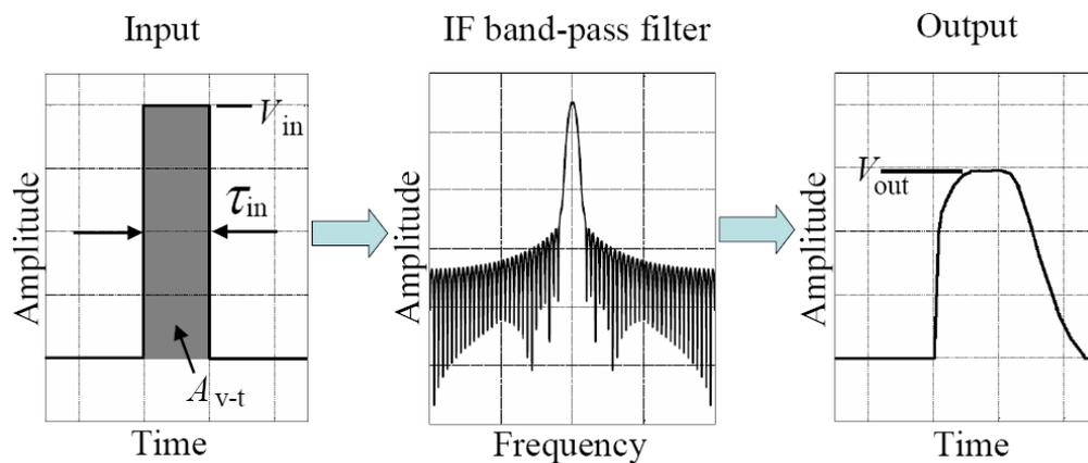
**Figure 5.16** Definition of the terms used in impulse bandwidth calculation.
