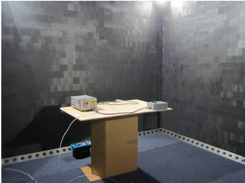
**Figure 8.1** Measurement setup in semi-anechoic chamber in the Finnish Army Materiel Command's EMC laboratory.
