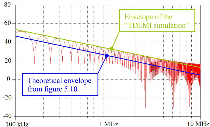
**Figure 5.12** Spectrum of a 4 kHz square wave signal. Simulated TDEMI measurement result for upper frequency band (150 kHz – 10 MHz).
