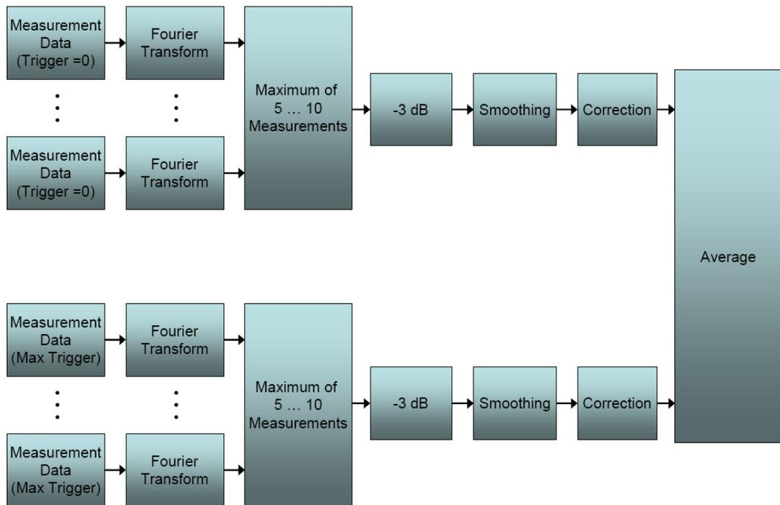
**Figure 1.3** Algorithm used in Keller's and Feser's paper *Fast Emission Measurement in Time domain* from 2001 [6].
