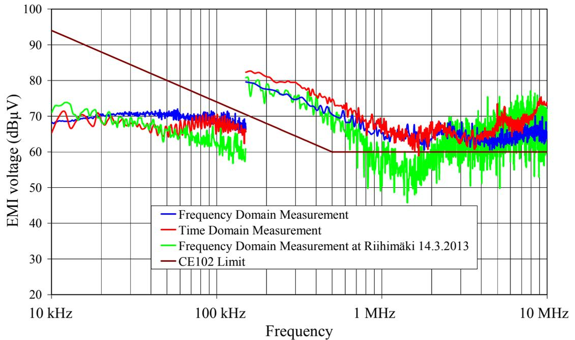
**Figure 8.2** TDEMI measurement results and frequency domain EMI measurement results, DC-motor of the reference EMI source, plus lead.
