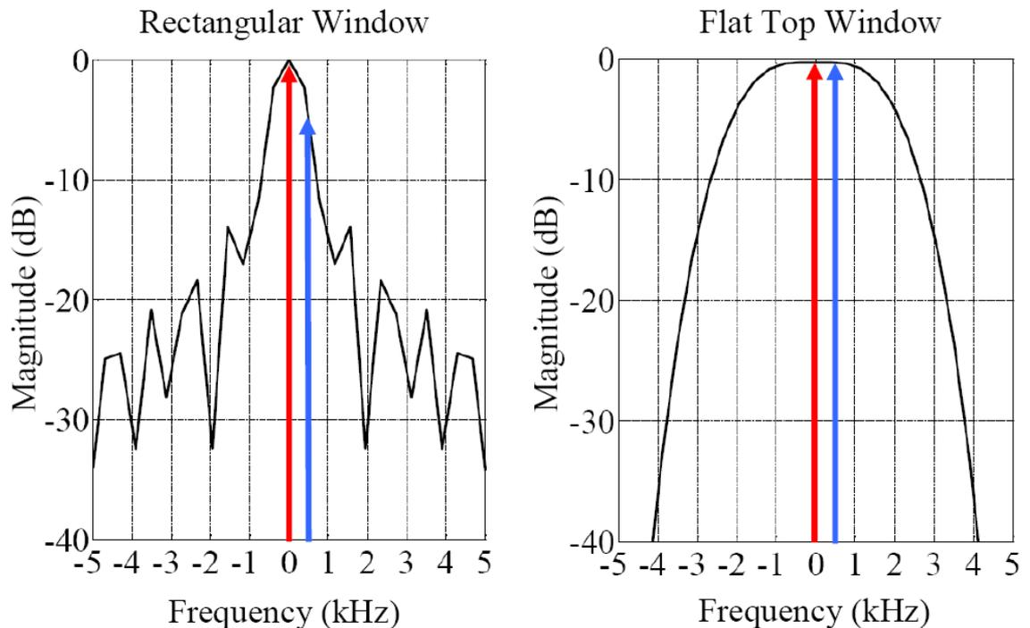
**Figure 5.3** Frequency responses of rectangular and Flat Top windows. Coherent gains are compensated.
