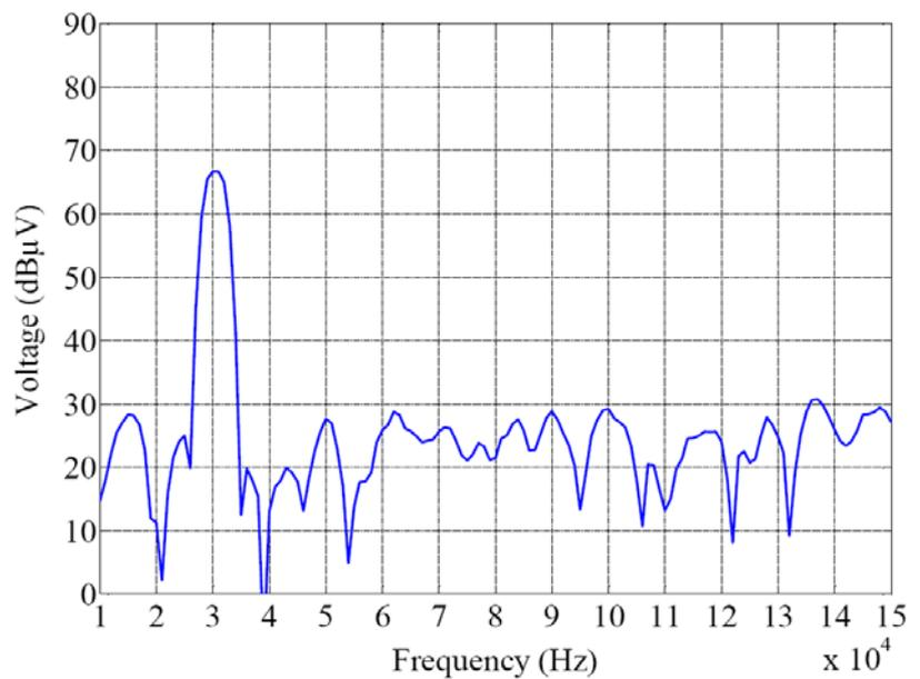
Amplitude spectrum of a 30.5 kHz sinusoidal signal with Flat Top windowing before DFT. Coherent gain compensated.
