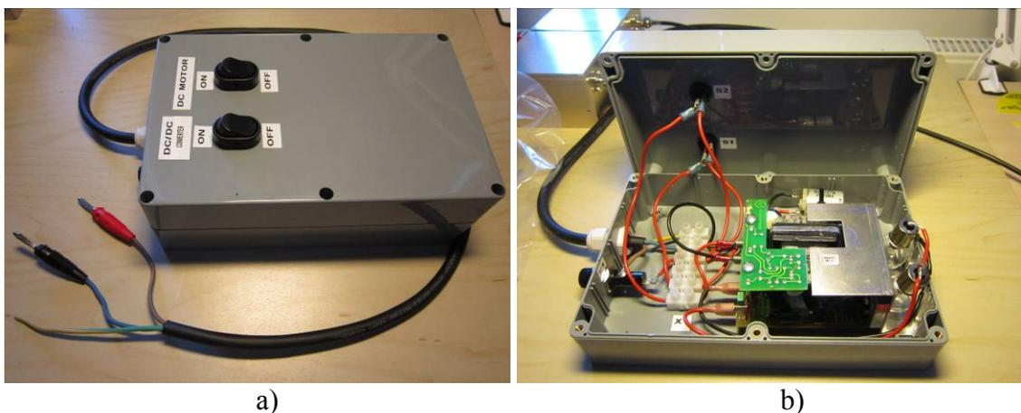
**Figure 3.7** a) The reference EMI source from outside b) The reference EMI source from inside.
