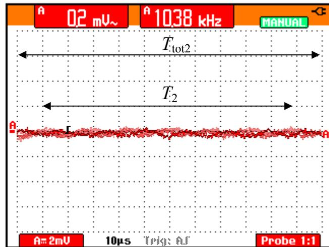
**Figure 4.3** Total capture time  $T_{tot2}$  and capture time  $T_2$  on frequency range 150 kHz to 10 MHz.  $T_2$  can be chosen arbitrarily from the  $T_{tot2}$ .
