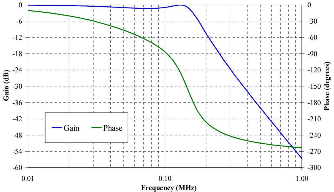
**Figure 4.6** Simulated gain and phase of low pass filter #1.
