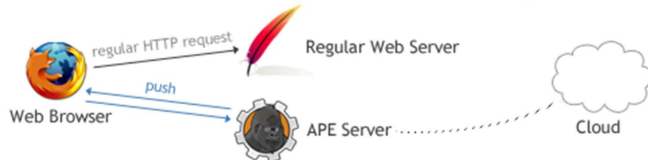
Figure 27: Ajax Push Engine (APE) working [51]
