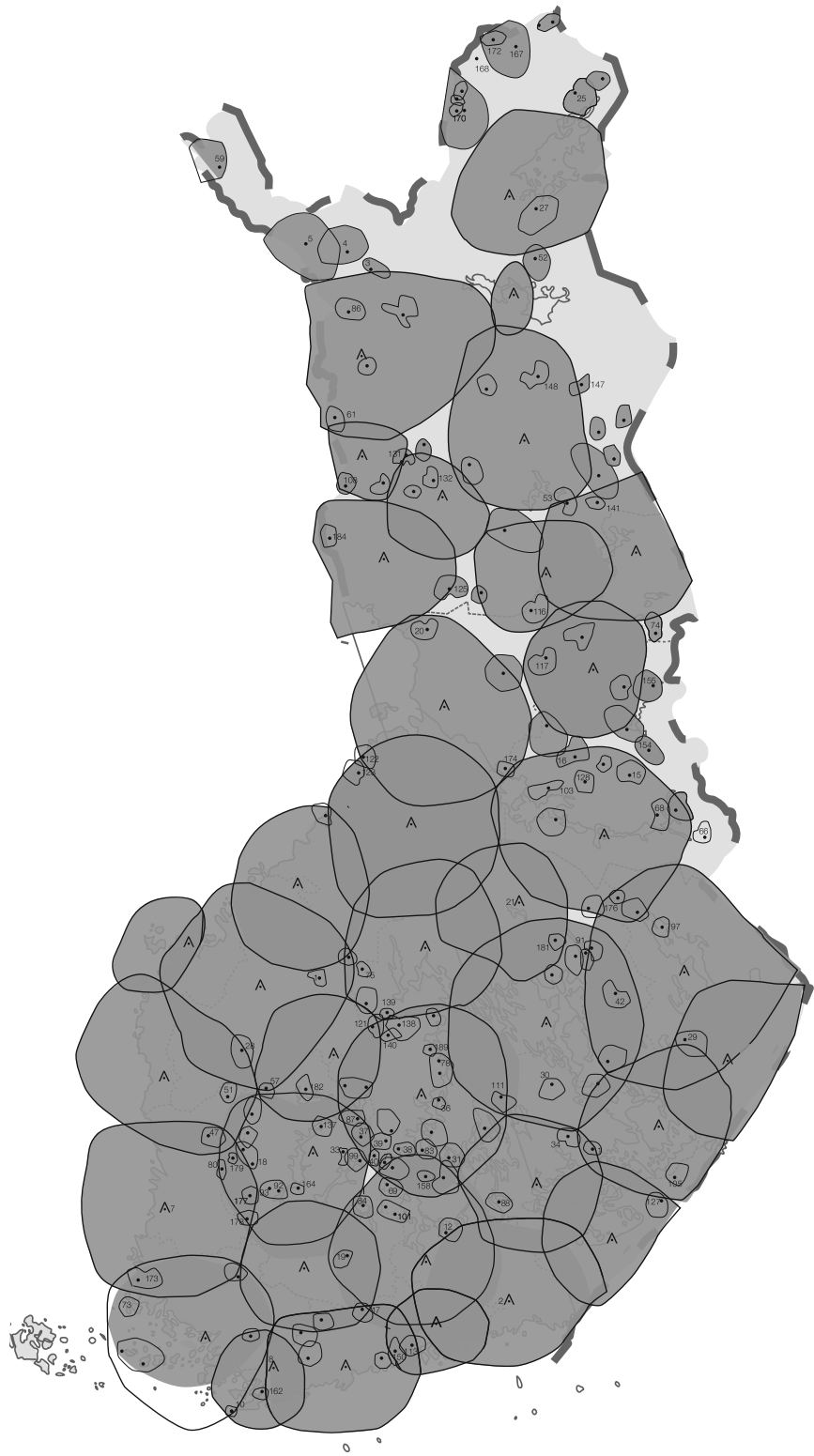
Figure 2.1: Approximate DVB-T coverage of Digitas's network. Each dot surrounded by a semi-circular coverage area is a transmitter. Adapted from [2] and [3]
