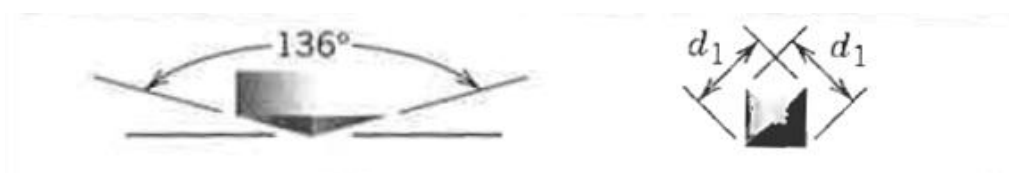
Figure 5.4. The shape of the diamond indenter used in Vickers hardness testing. [5]
