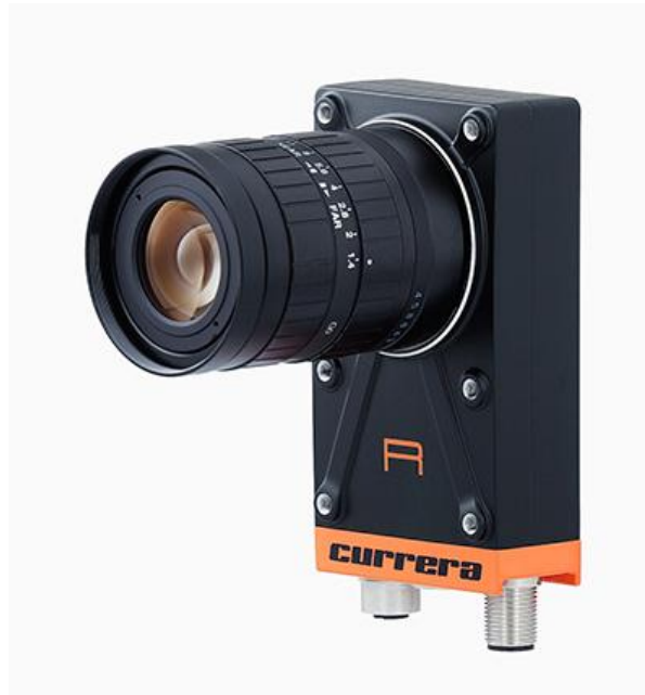
Figure 4.12. Currena RL50C smart camera. [44]
