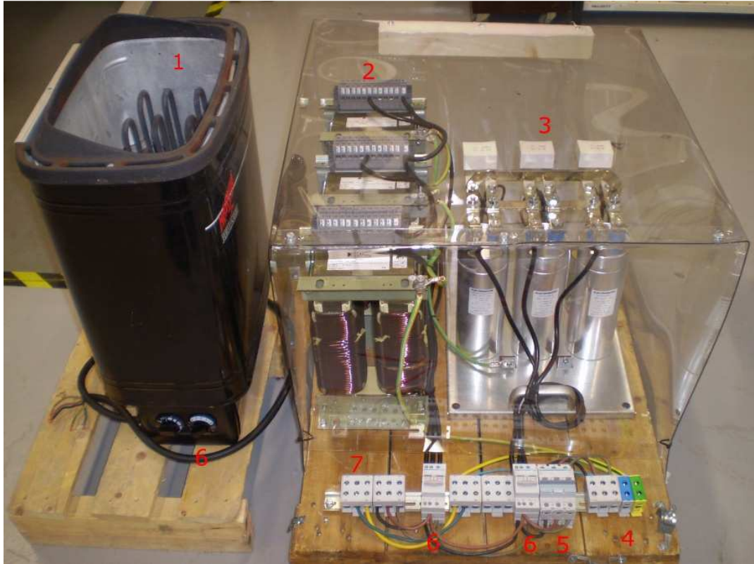
Figure 4.2. Parallel RLC load for islanding testing.
