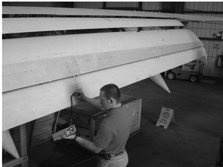
Figure 2-1. Traditional inspection of the composite structures. [6]
