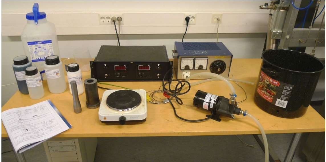
Figure 3.8. Facilities for application of electroless nickel coating with boron nitride particles.
