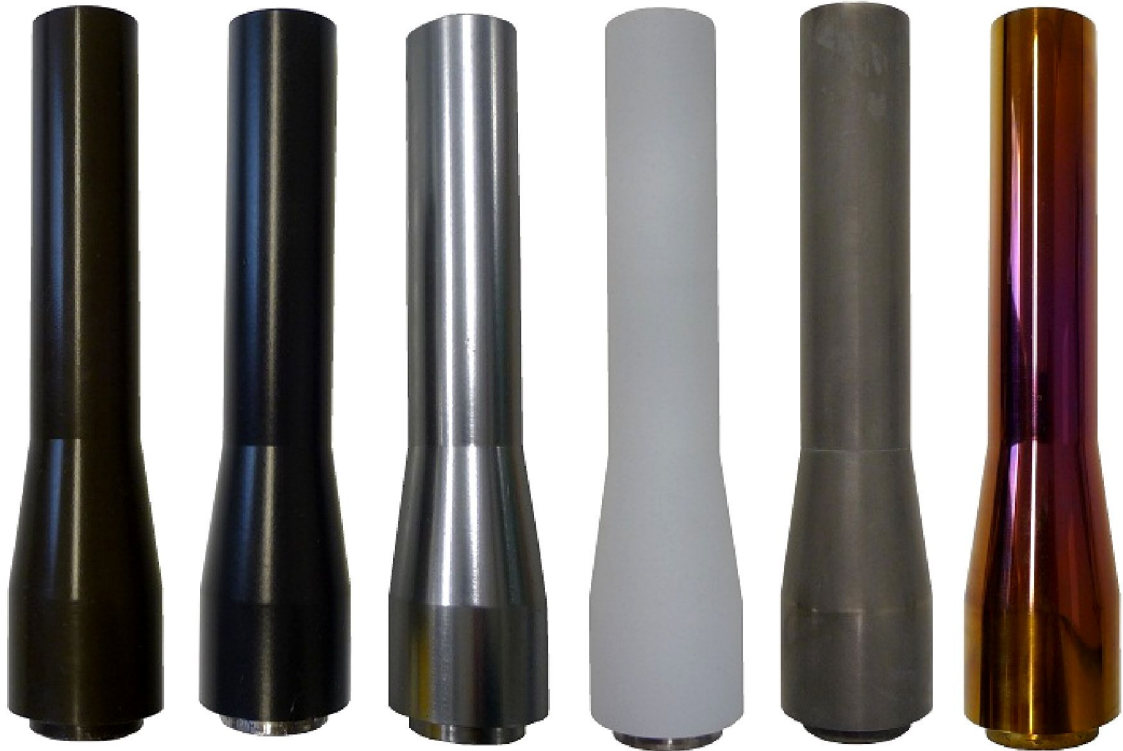
Figure 3.7. Coatings on the surface of torpedo from left to right: fluoropolymer coatings 1 and 2, hard chrome plating with fluoropolymer (3), boron nitride (4), boron nitride electroless nickel (5), and metal oxide (6).
