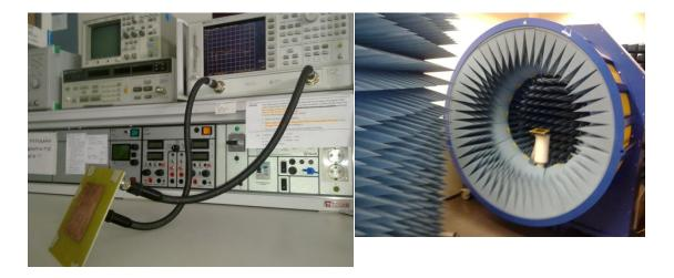
Fig. 7.6 Measurement set up for S parameters by VNA (left) and Satimo Starlab (right)
