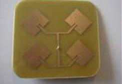
d) Feeding separate patches using a power dividing circuit [41]
