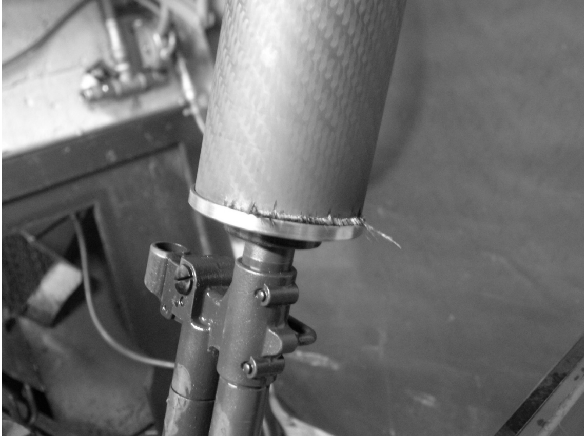
Figure 26 Damage caused to the suppressor outer shell by propellant gas leak between the end cap and outer shell.
