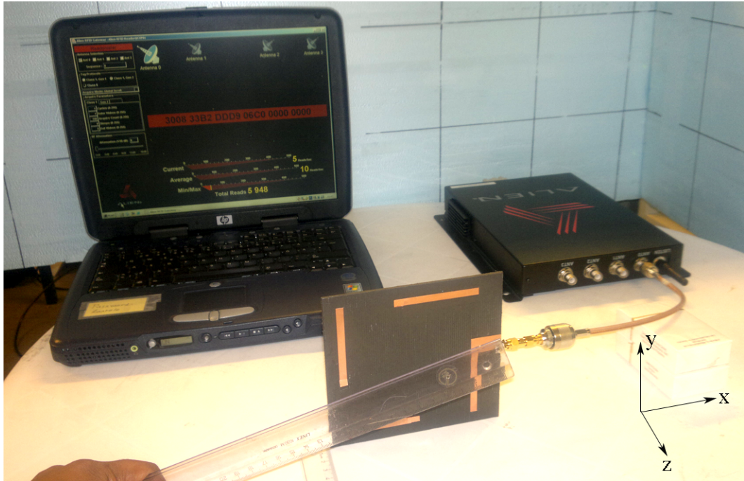
Figure 6.16: Measurement Set Up for Reading Performance.
