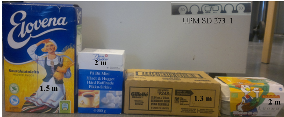
Figure 6.19: Read-Range for Far-Field Measurements With Objects.
