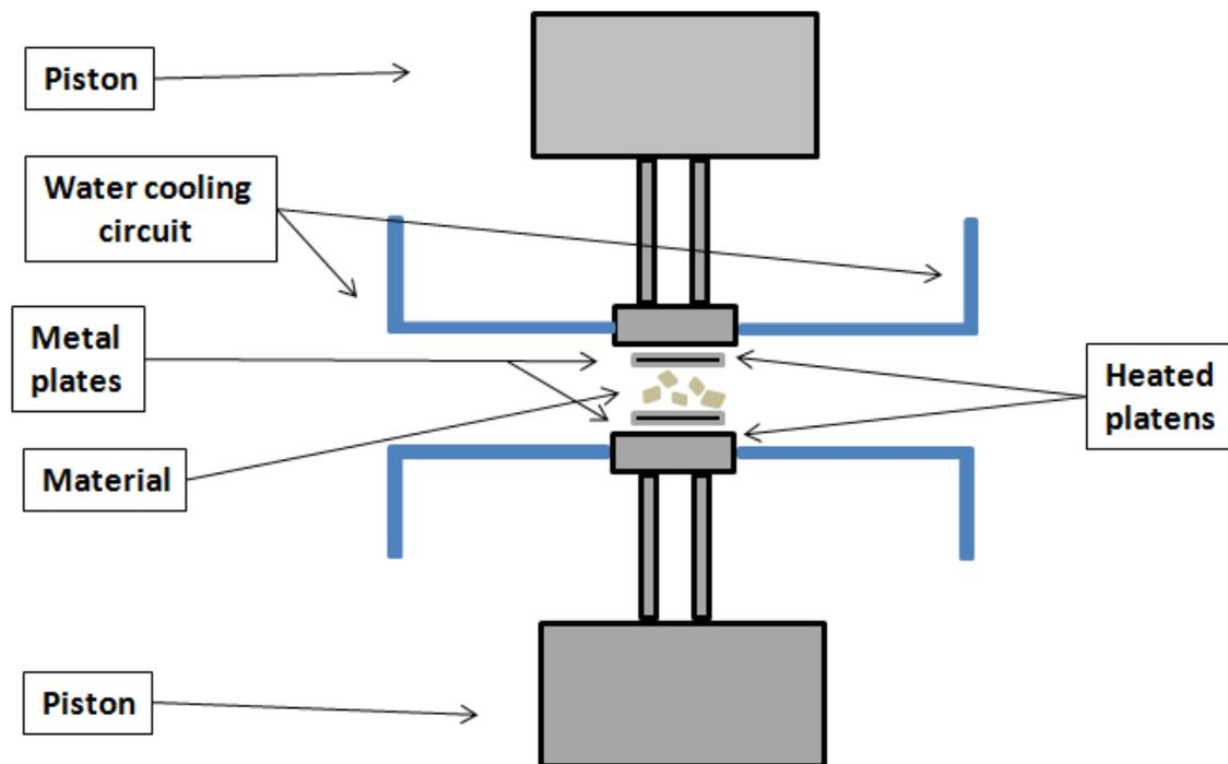
**Figure 8.3** Compression molding equipment and conditions.
