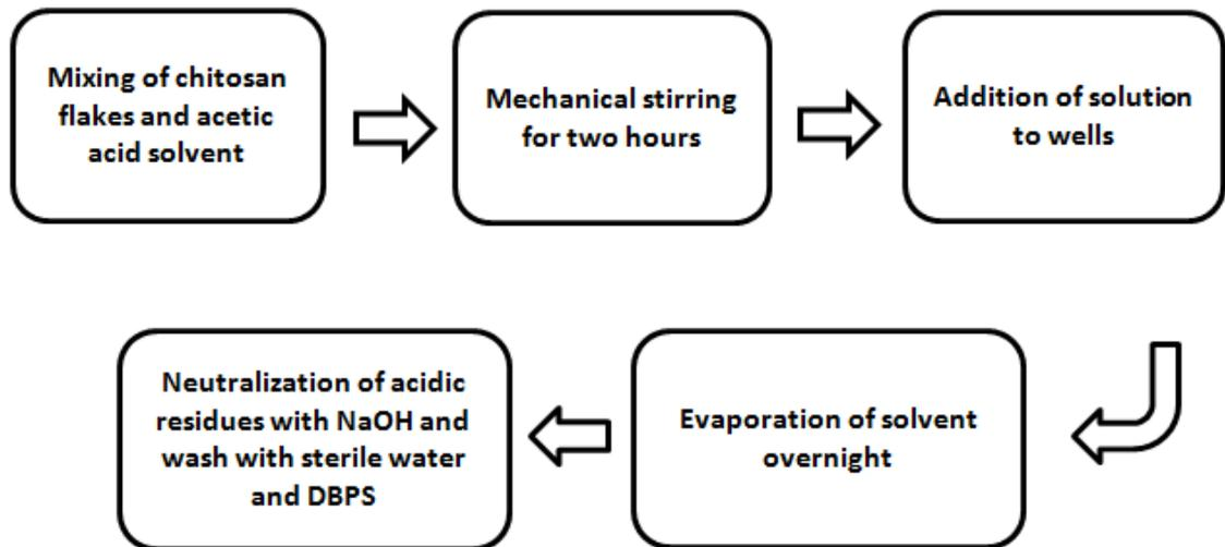
**Figure 8.2.** The schematic figure of solvent casting method applied to produce chitosan coatings.
