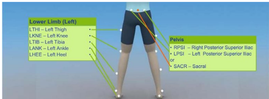
Figure 6: Backview of marker placement for lower body (Vicon Motion Systems Ltd., 2010, p. 12).
