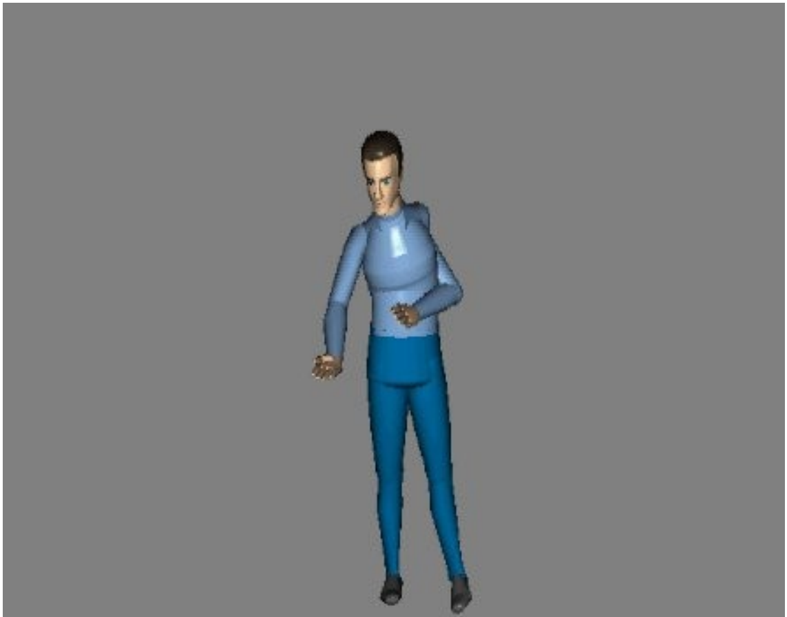
Figure 13: Motion capture data from the manual task was sent to the virtual environment, where they controlled a digital human model. Due to stability issues in motion capture the models segments did not precisely meet the reality.
