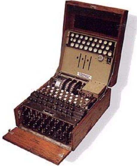
**Figure 9. Germany's Enigma - Rotor based substitution cipher machine**
