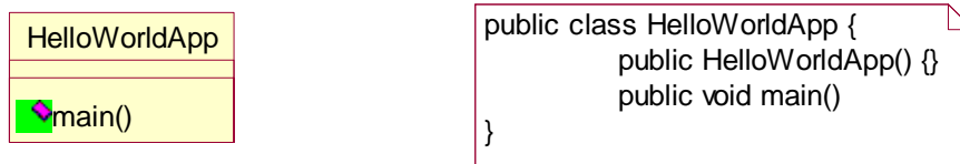
Figure 15. Java methods and the mapping to UML.
