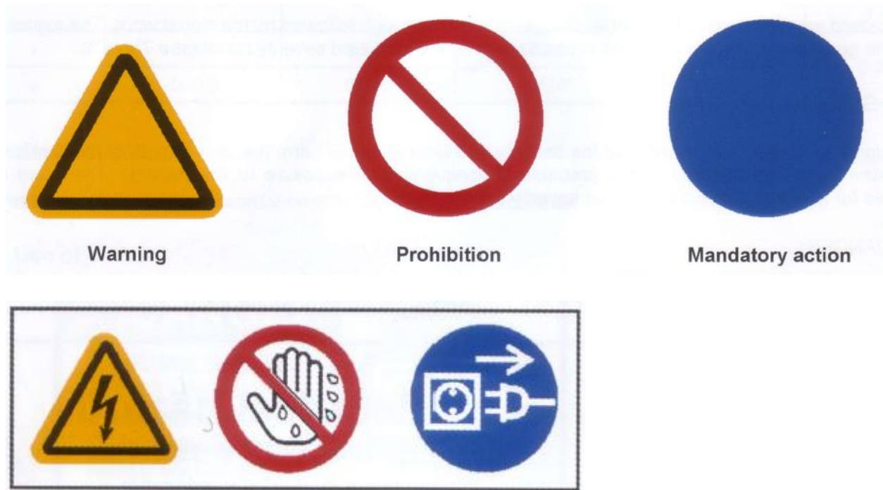
Fig. 1. The three safety sign categories and an example of each.
