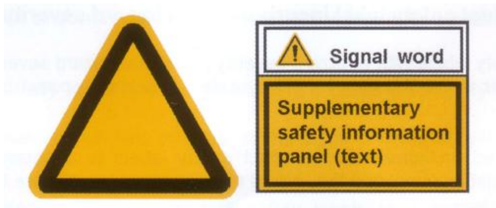
Figure 11. Type c): single safety sign used with a separated supplementary safety information text panel which includes a hazard severity panel (ISO 2004, 6).
