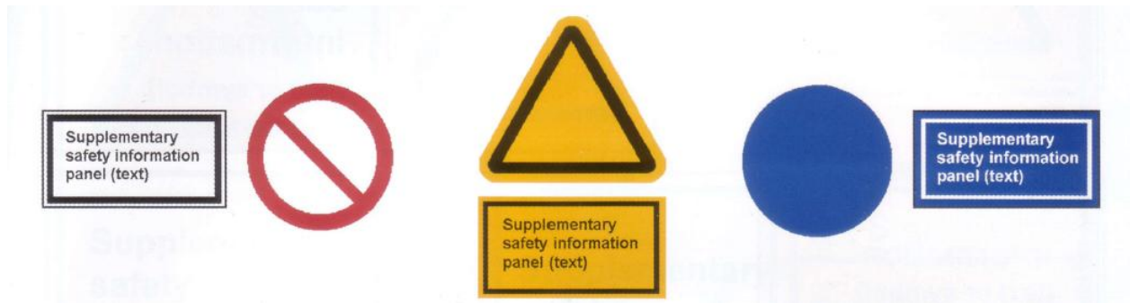
Figure 10. Type b): single safety sign used with a separated supplementary safety information text panel (ISO 2004, 6).
