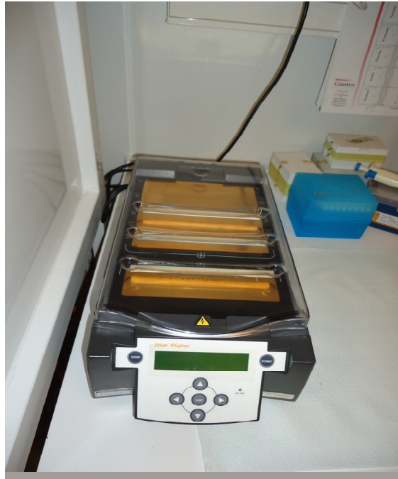
Figure 1: Ettan IPGphor. Differently charged proteins can be separated by this machine on the basis of their isoelectric points by using an immobilized pH gradient strip
