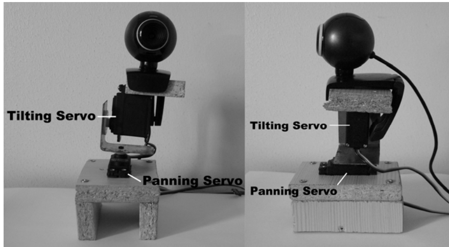
Figure 4-5 A photo of the motorize web-camera setup. Note: the slating was a result of a transportation accident. When the experiment was carried out there was no tilting of the apparatus.
