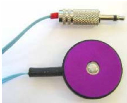
Pictur 5 C2 tactor, which is a widely used linear vibration motor [Brown et al., 2005]
