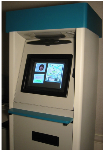
Figure 4.6: MATCH Kiosk Hardware which responds to both touch and speech [42].
