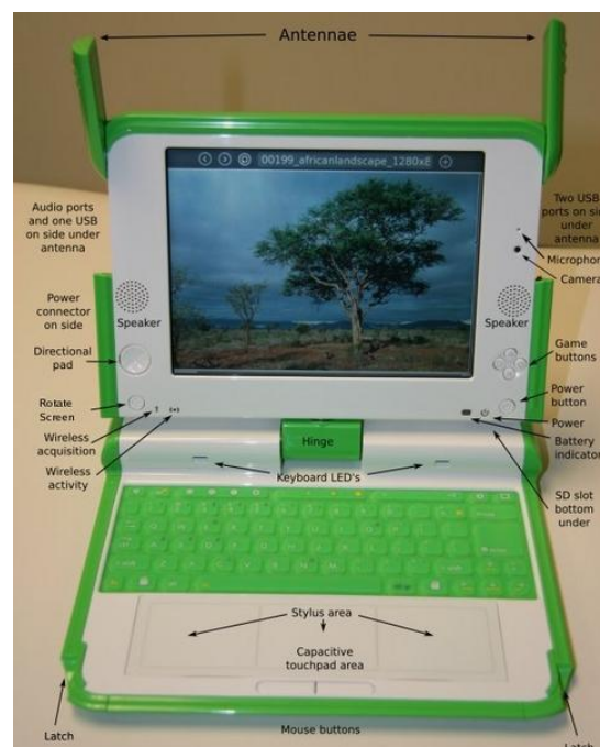
Figure 11: OLPC XO laptop with labels [OLPC wiki, 2007].
