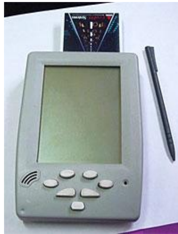
Figure 4: The early design of Simputer [Simputer Trust, 2000]
