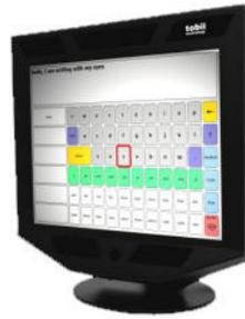
**Figure 2.** Tobii 1750 eye tracker integrated with 17" TFT display
