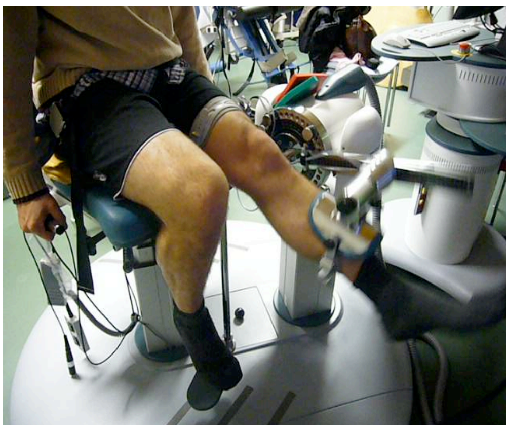
Figure 4. The patient strapped to the muscle strength testing apparatus. Five maximal repetitive knee flexion-extension movements were performed.
