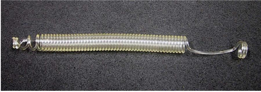
Figure 3. PLGA 80/20 prostatic stent
