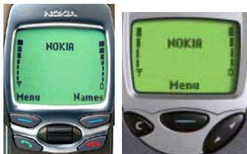
*Figure 4.4.* Nokia 7110 (left) has two softkeys and a “roller” for UI navigation. Call handling keys are green and red buttons. Nokia 3110 (right) has one softkey and up/down arrows for navigation. No special keys for call handling.
