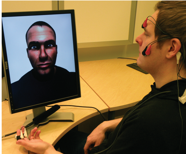
Fig. 3. The first author seated at a distance of 50 cm from the monitor while wearing the EMG and EDA electrodes.
