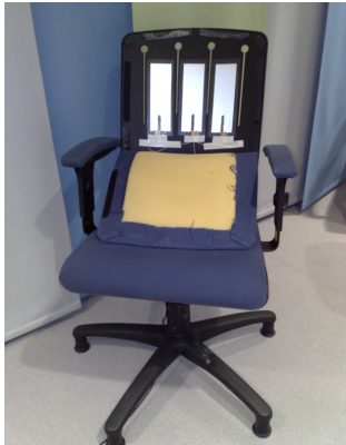
Figure 1. The EMFi chair. The back rest contained three strips of electromechanical film (EMFi). The back cushion is folded and the sensors are revealed for demonstration.
