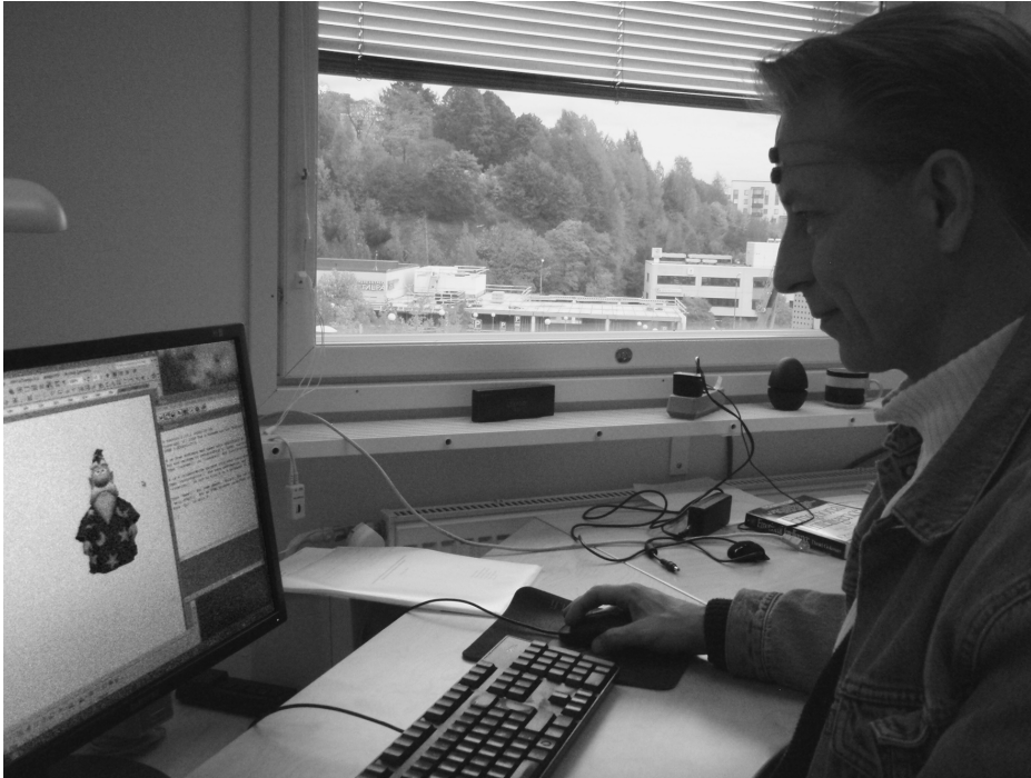
Figure 9.1 A person interacting with a software agent. This agent records the changes in the level of electrical facial muscle activities, and interprets these activations with the help of signal-processing algorithms. In the prototype, a software agent can be called on for help by raising the eyebrows (a common gesture when one is faced with problems or surprises). This agent can be forced to disappear by lowering the eyebrows (a common gesture used for expressing a negative attitude).
