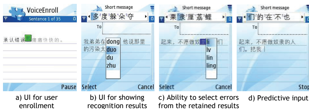
Figure 5.2. The screenshots for the isolated Mandarin message dictation application on a Symbian S60 phone.
