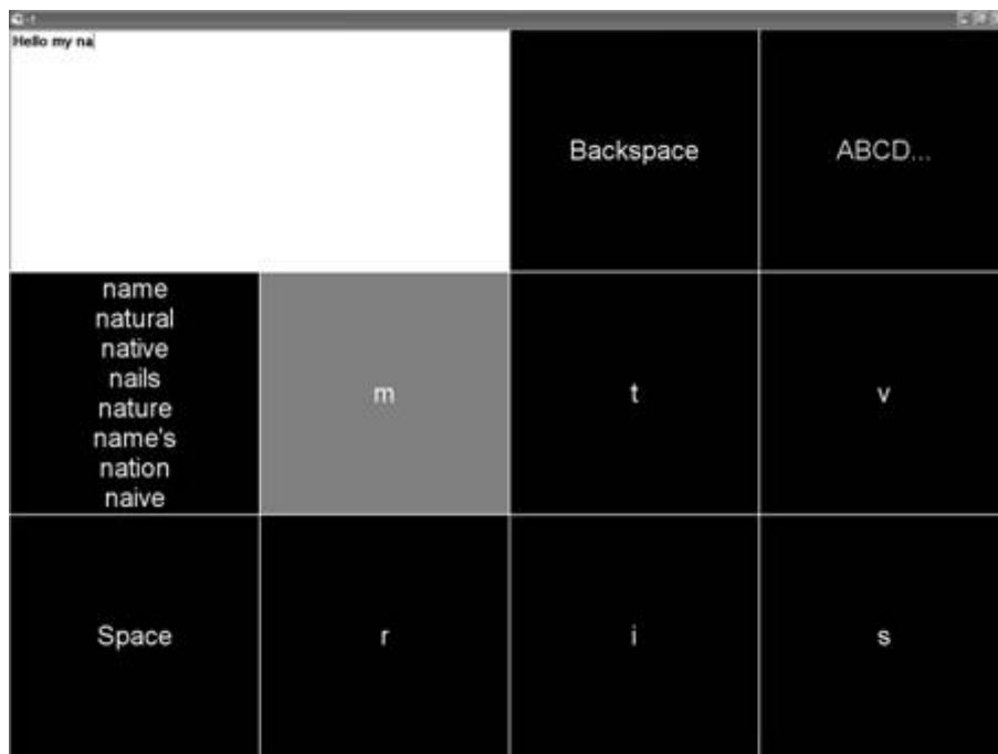
Figure 5.2. GazeTalk 13 (Hansen et al., 2001) provides big buttons that are easy to hit. To speed up typing, it provides a list of the next probable words, predicted on the basis of the text written so far. If the user selects the cell with the list of words, the cells that now contain individual letters will be filled in with the words.
