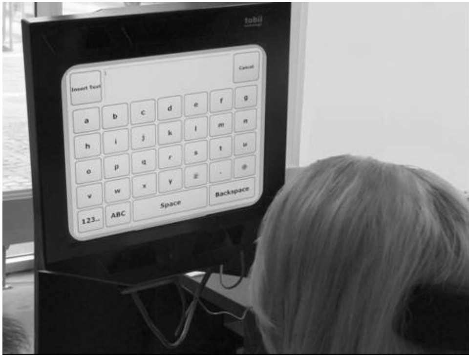
Figure 5.1. The Tobii eye tracking device has a camera integrated into the frame of the monitor that shows the on-screen keyboard (photo: Henna Heikkilä).
