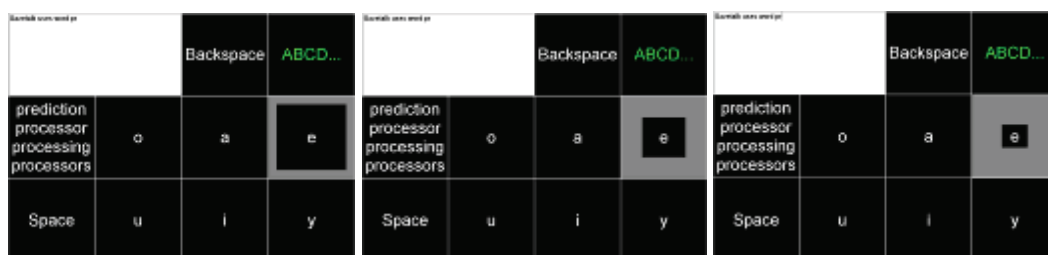
Figure 8.1. GazeTalk provides visual feedback on the dwell time progress for the letter “e.”
