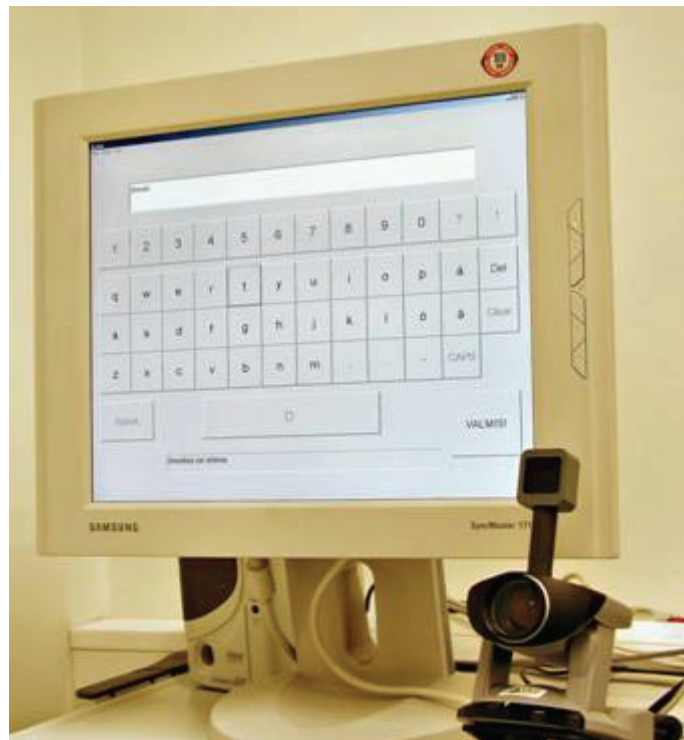
Figure 8.2. Experimental setup: on-screen keyboard and eye tracking device.
