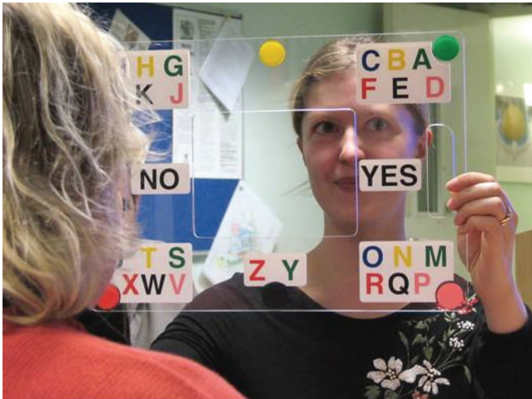
Figure 4.1. A gaze communication board (“E-Tran frame”). The person on the other side of the board acts as a human eye tracker and interprets the direction of gaze through the transparent board. A letter is chosen by first looking at it and then looking at the color button that corresponds to the color of the letter. 6
