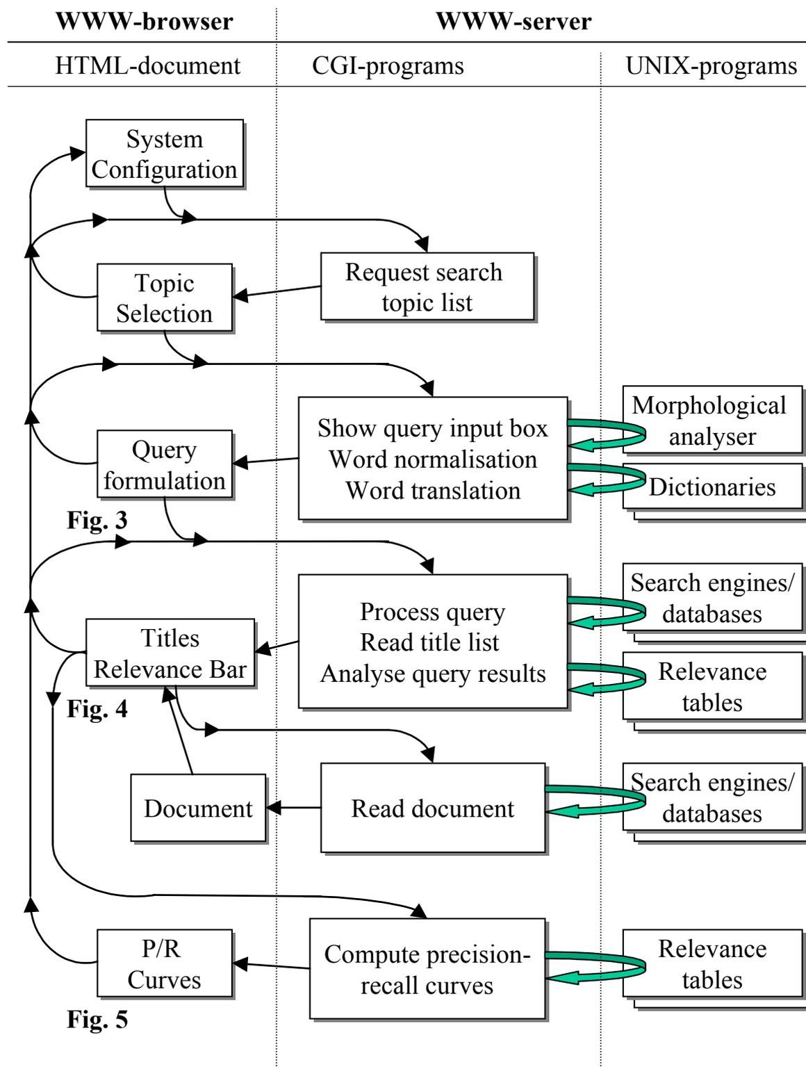
Figure 2. General view of the flow of operation in the Query Performance Analyser, version 3.5.
