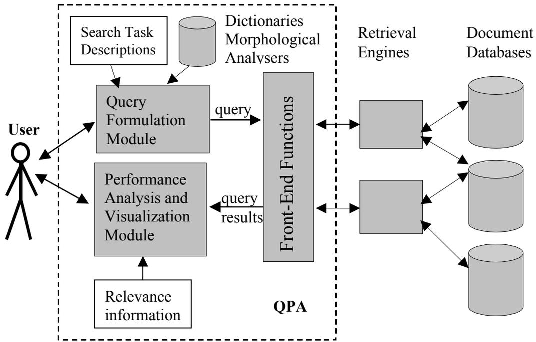
Figure 1. The basic functional components of the Query Performance Analyser.
