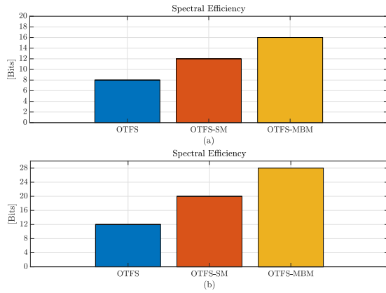
Fig. 3. Spectral efficiency comparisons of the proposed OTFS-MBM, OTFS-SM, and OTFS systems for (a) M_q = 4 , N_T = 2 , n_{RF} = 2 and (b) M_q = 8 , N_T = 4 , n_{RF} = 4 .
