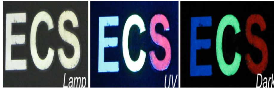
Figure 10. Three-color persistent luminescence panel based on the \text{Sr}_2\text{MgSi}_2\text{O}_7:\text{Eu}^{2+}, \text{Dy}^{3+} (blue), \text{SrAl}_2\text{O}_4:\text{Eu}^{2+}, \text{Dy}^{3+} (green), and \text{Y}_2\text{O}_2\text{S}:\text{Eu}^{3+}, \text{Mg}^{2+}, \text{Ti} (red) phosphors (Brito,12)
