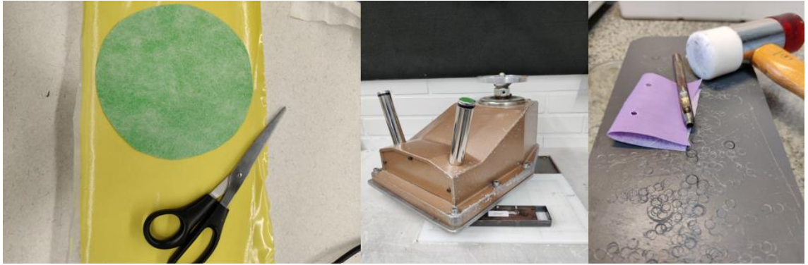
Figure 14. Obtaining of water vapor permeability test, tensile test and DSC samples, respectively.
