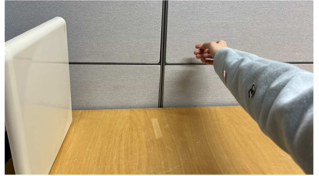
Fig. 4. Direction for radiation exposure. The sleeve was dressed on and arm held extended while exposed to radiation. Both dipole antennas are in upright position.
