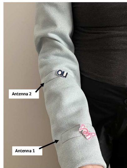
Fig. 5. The ready-made command sleeve with two antennas and two output markers with microcircuits underneath
