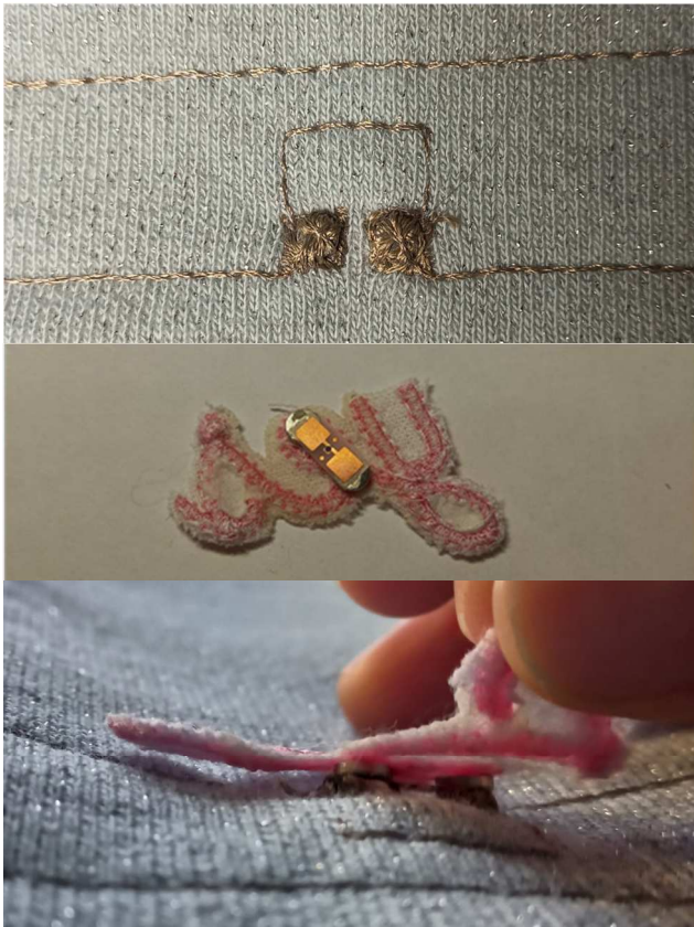
Fig. 3. Changeable IC+magnet structure: first, a magnet pair was stitched by hand onto antenna bedding (top); second, the other magnet pair was glued to IC and to output marker (middle); last, the IC+magnet pair was placed to antenna embroidered to sleeve (bottom).
