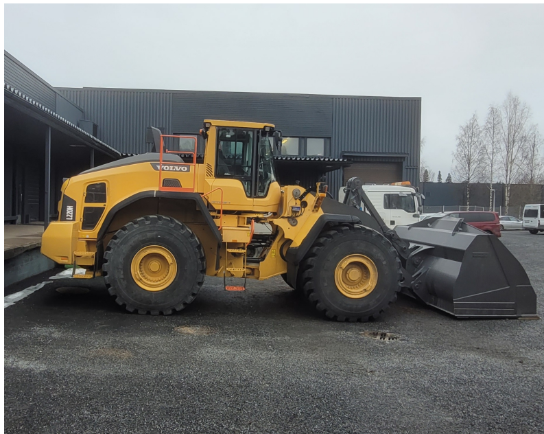
Figure 3.1. Volvo L220 wheel loader used for data collection
