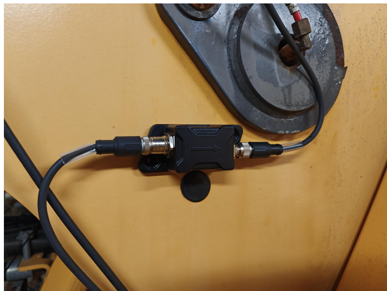
Figure 3.2. IMU sensor attached to the body of the wheel loader
