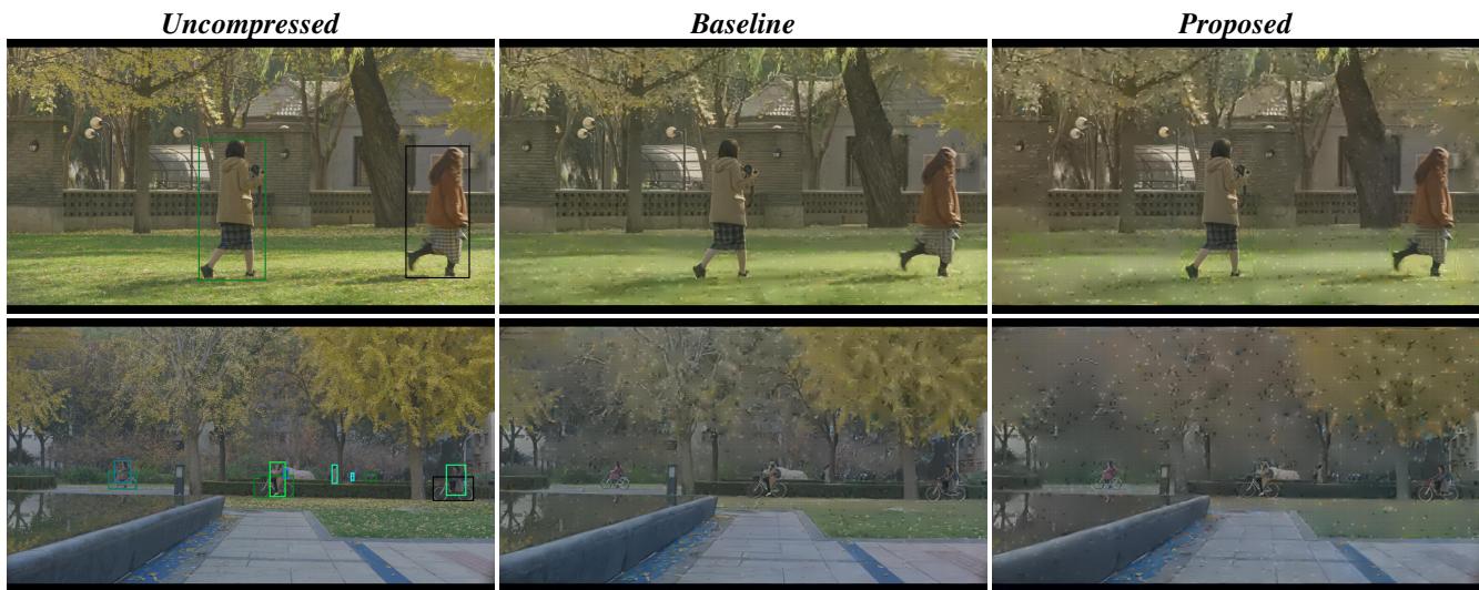
Fig. 5: Encoded images of the proposed ROI LIC method compared against the baseline LIC model on QP 42. Predicted bounding boxes used with the proposed method are shown on top of the uncompressed input images.
