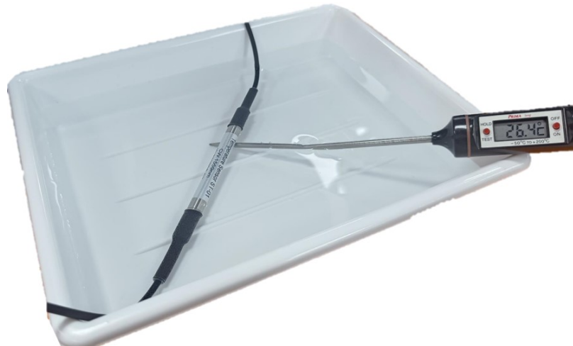
Figure 5.1. Temperature measurement setup for commercial sensor
