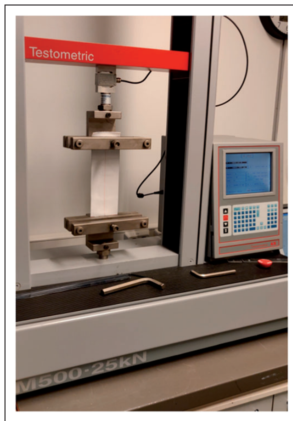
Figure 1. Elastic band stretch test measurement setup.
