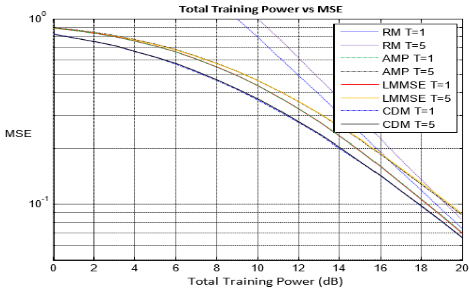
Figure 10: Total Training Power versus MSE for a massive MIMO system compared to different methods RM, AMP, LMMSE, and CDM
